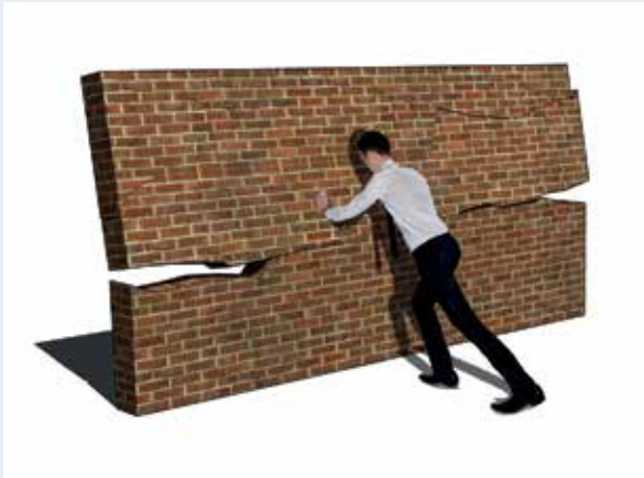
(a) Schematic of a wall responding out-of-plane
