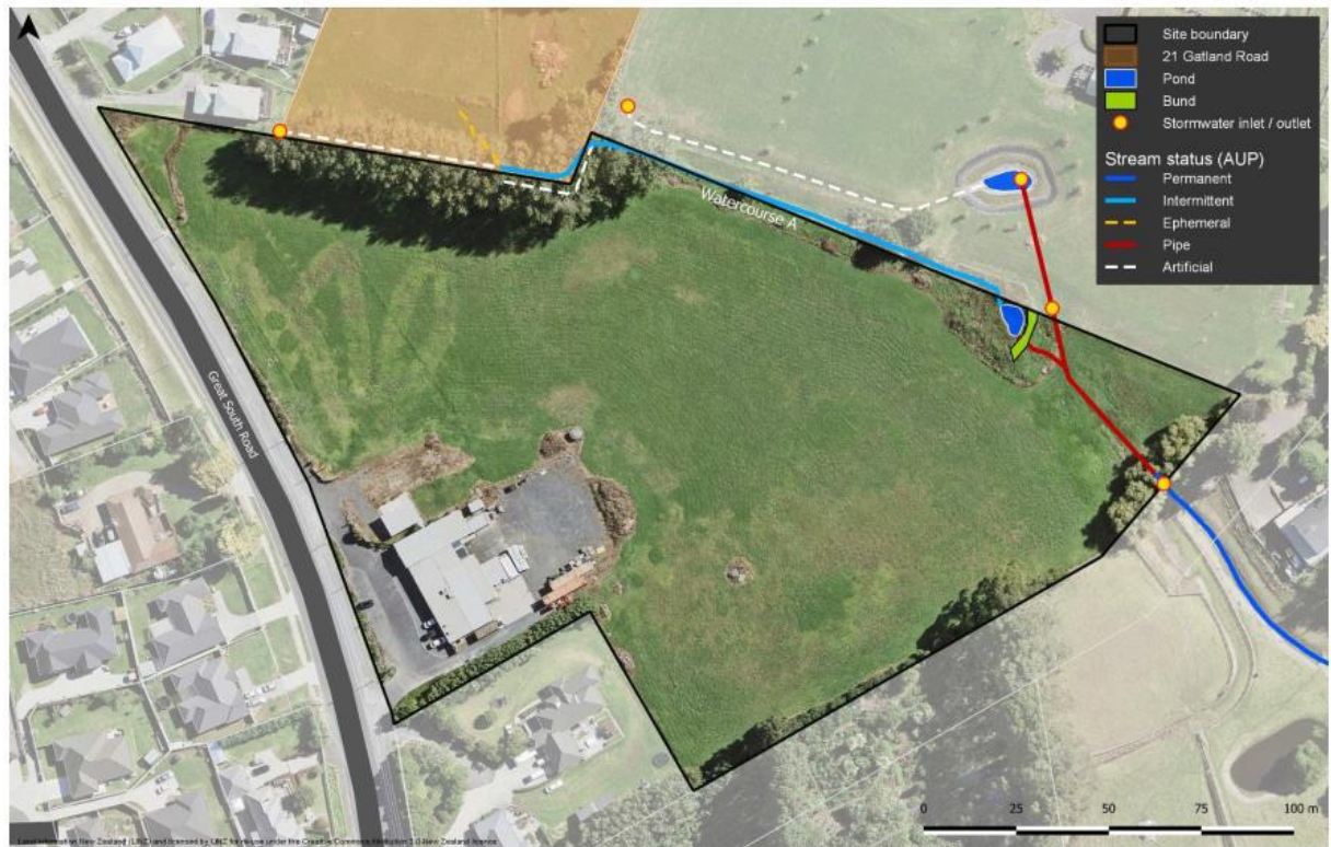
Figure 11: Alignment of Watercourse A and piped infrastructure on 520 Great South Road (Figure 2-8, SMP)
