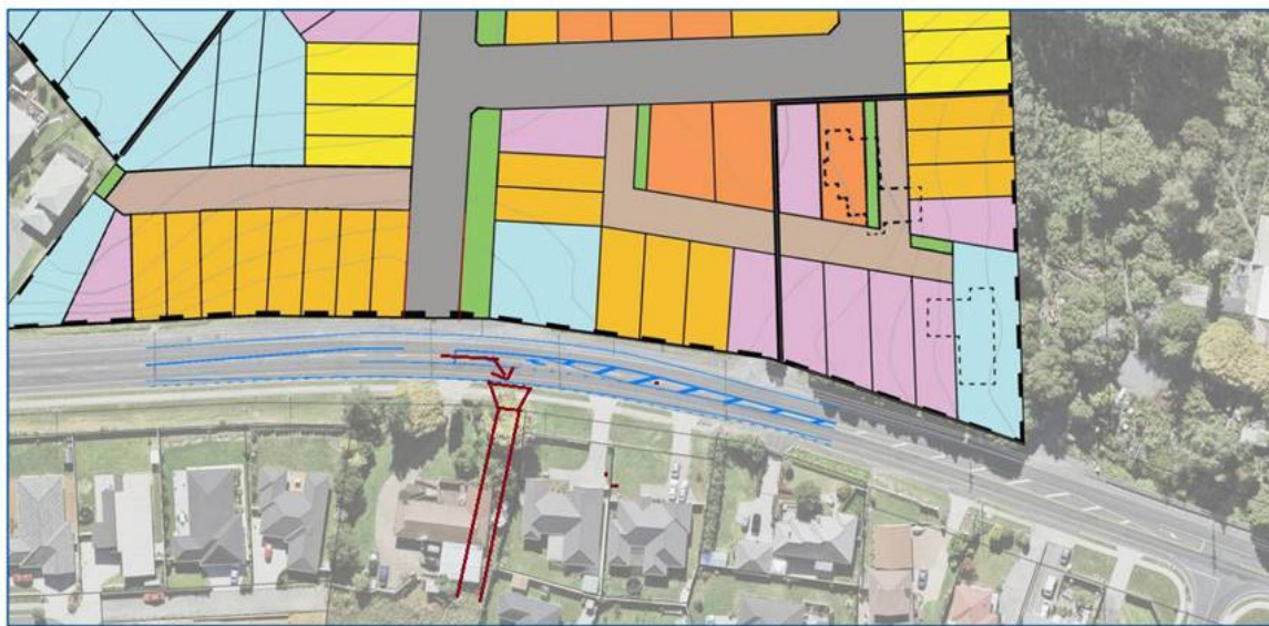
Figure 8 Proposed intersection on Great South Road - concept layout
