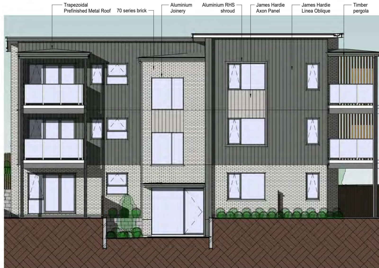
1 Type Lot 42 Apartments - East Elevation 1 : 100
