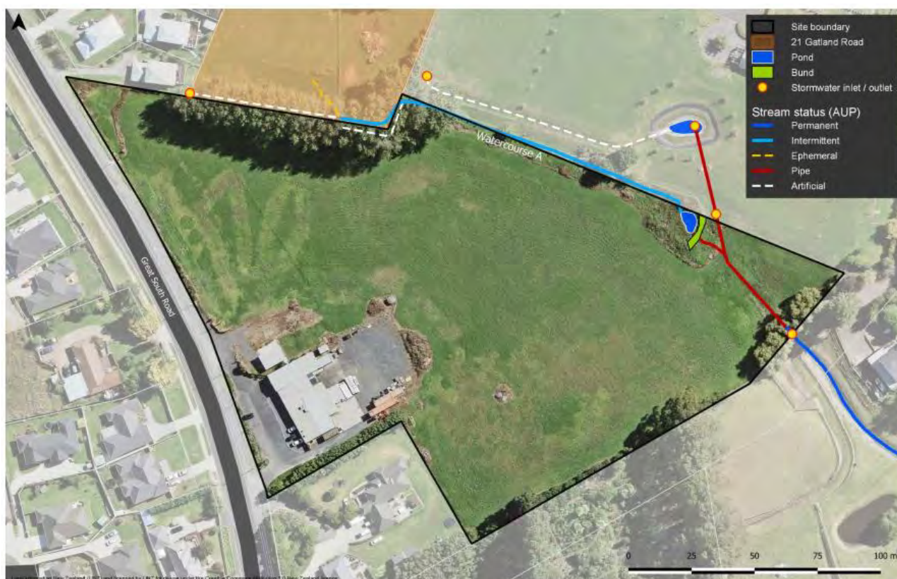
Figure 2-8: PCA existing private stormwater drainage (Freshwater Solutions, 2020)
