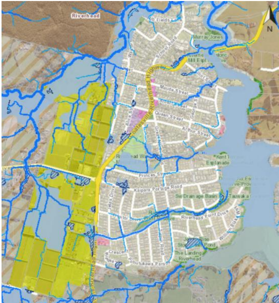
Figure B: 1% AEP floodplain and overland flow path over the PPC 100 site (highlighted in yellow) and in the surrounding area as shown on GeoMaps.
