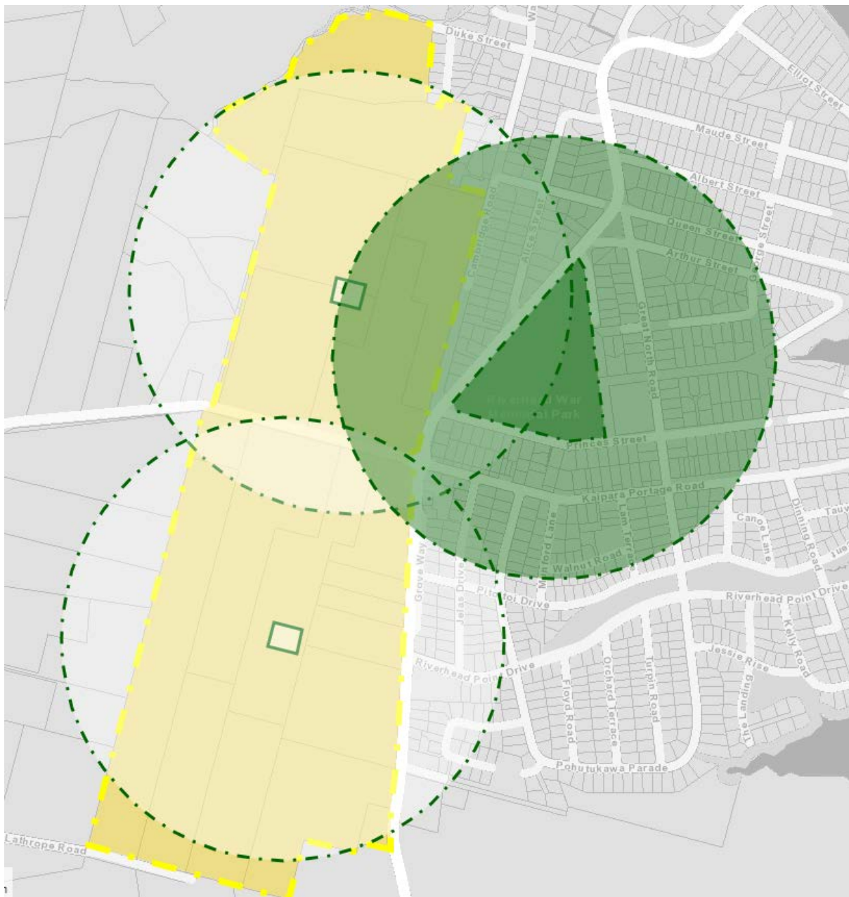
Figure 14: ‘Pedestrian shed’ analysis best locations for two additional parks for PC100 precinct plan purposes with no multi-purpose green corridor (Source: Rahman Bashir – Principal Property Provision Specialist)
