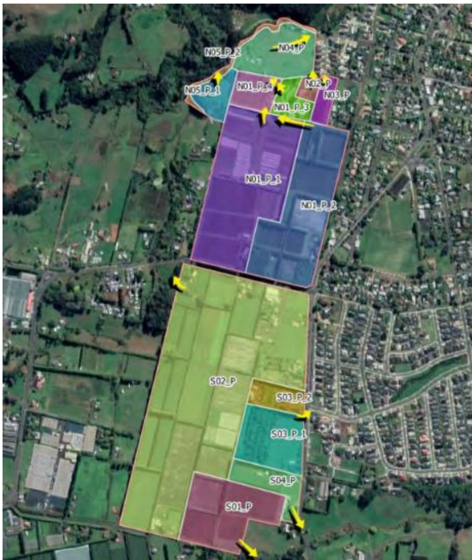
Figure 11 in the SMP showing the proposed sub-catchments with PPC 100 and indicative discharge locations.
