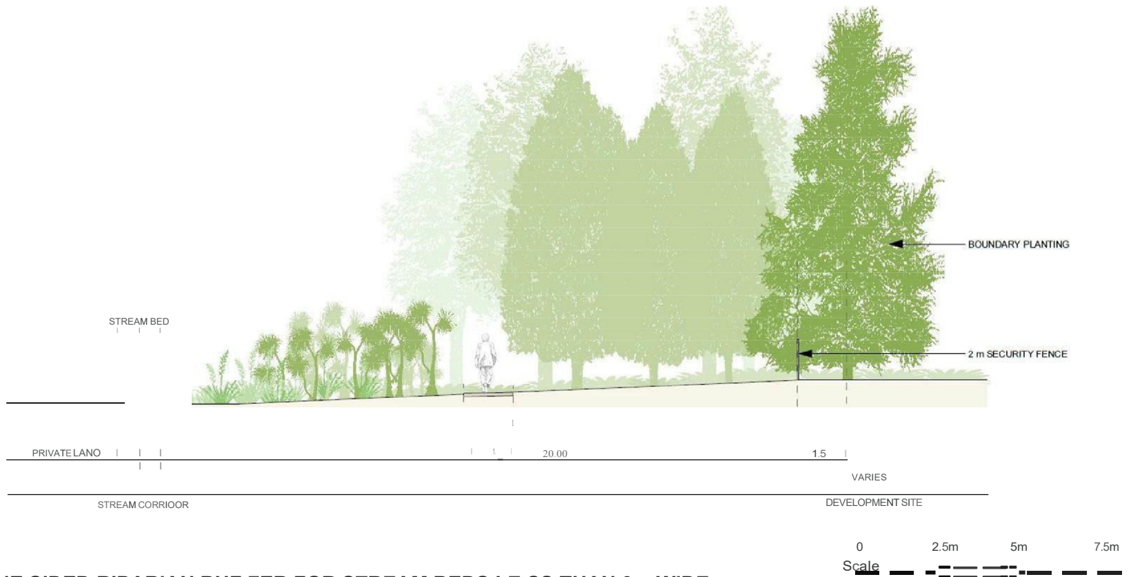
TYPICAL ONE SIDED RIPARIAN BUFFER FOR STREAM BEDS LESS THAN 3m WIDE
