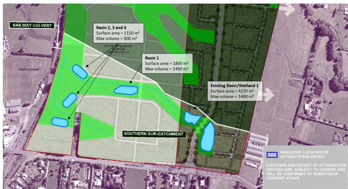
Figure 2: Indicative attenuation device locations within the southern sub-catchment of the Waihoehoe PCA
