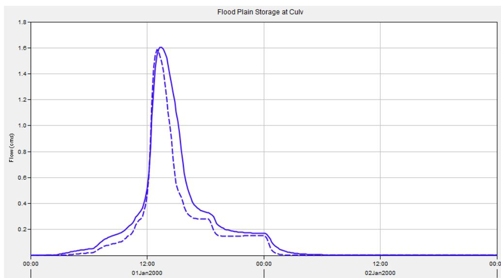
Figure 6: Peak flowrates at the railway culvert within the Downstream sub-catchment. Dashed line = pre-development scenario and the solid line = post-development scenario.
