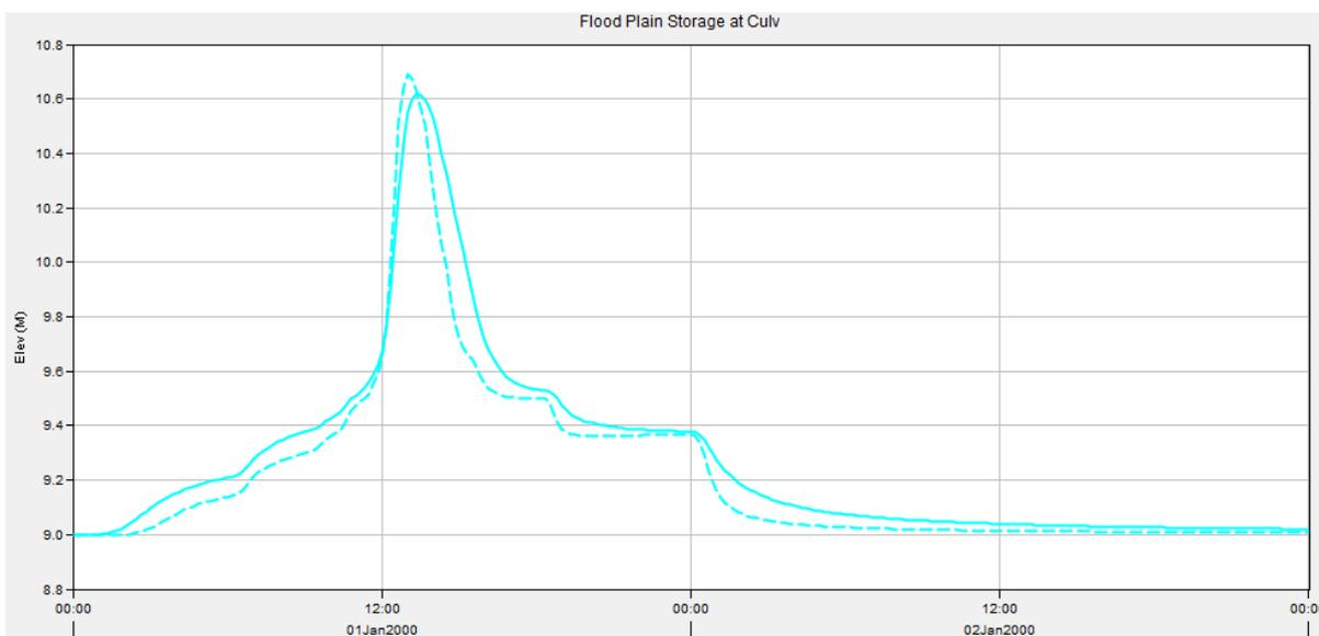
Figure 8: Peak water levels within the southern sub-catchment floodplain upstream of the railway culvert. Dashed line = pre-development scenario and the solid line = post-development scenario.
