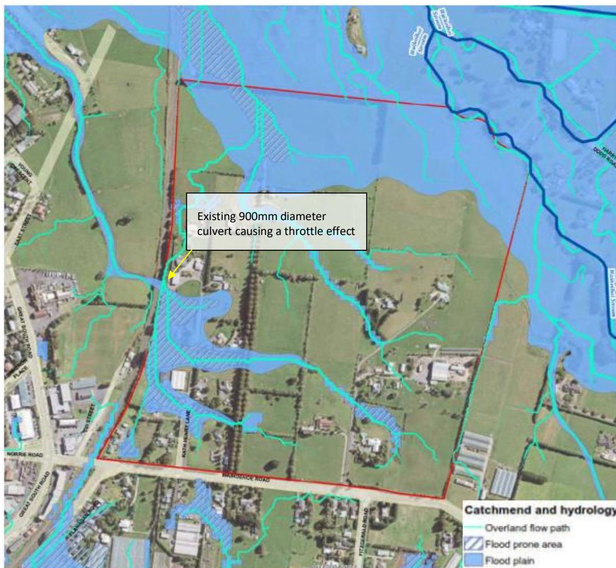
Figure 1: Flooding and overland flow paths within the Waihoehoe Precinct and railway culvert
