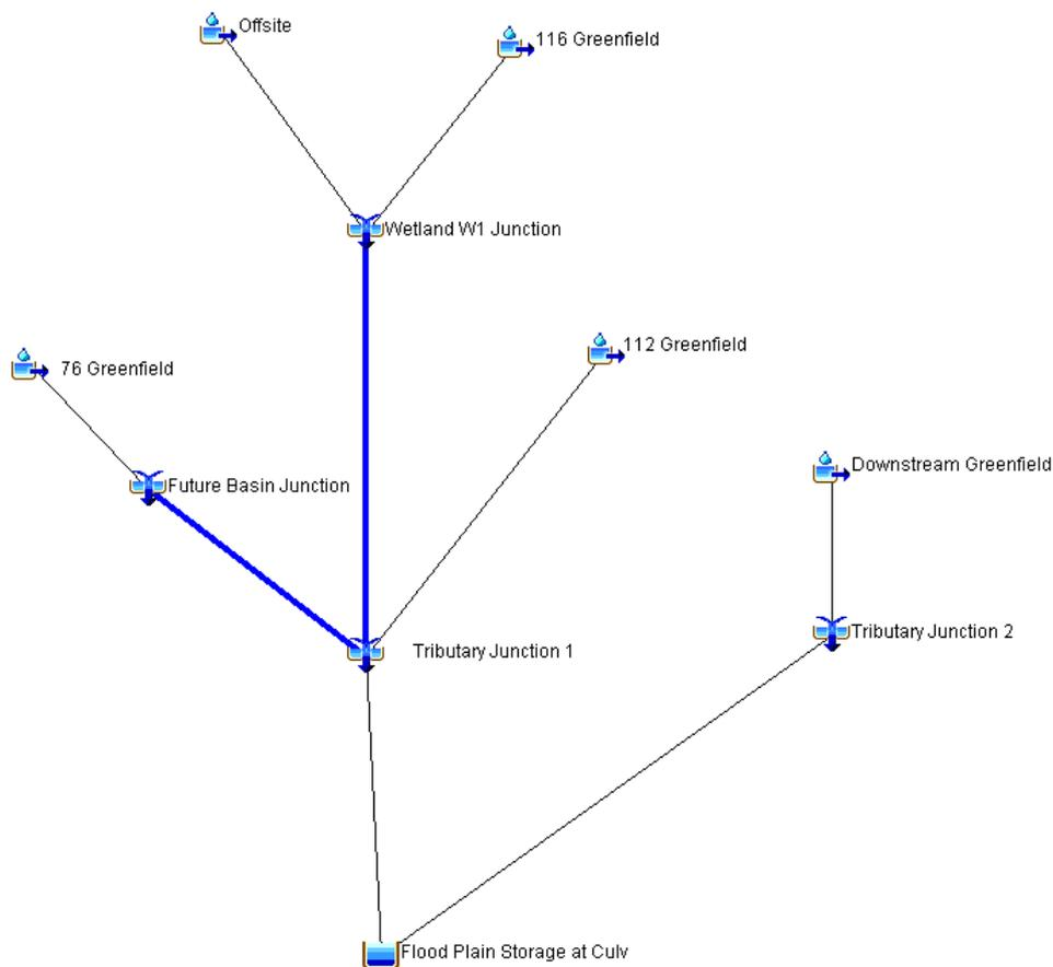
Figure 4: Pre-development basin model layout within HEC-HMS
