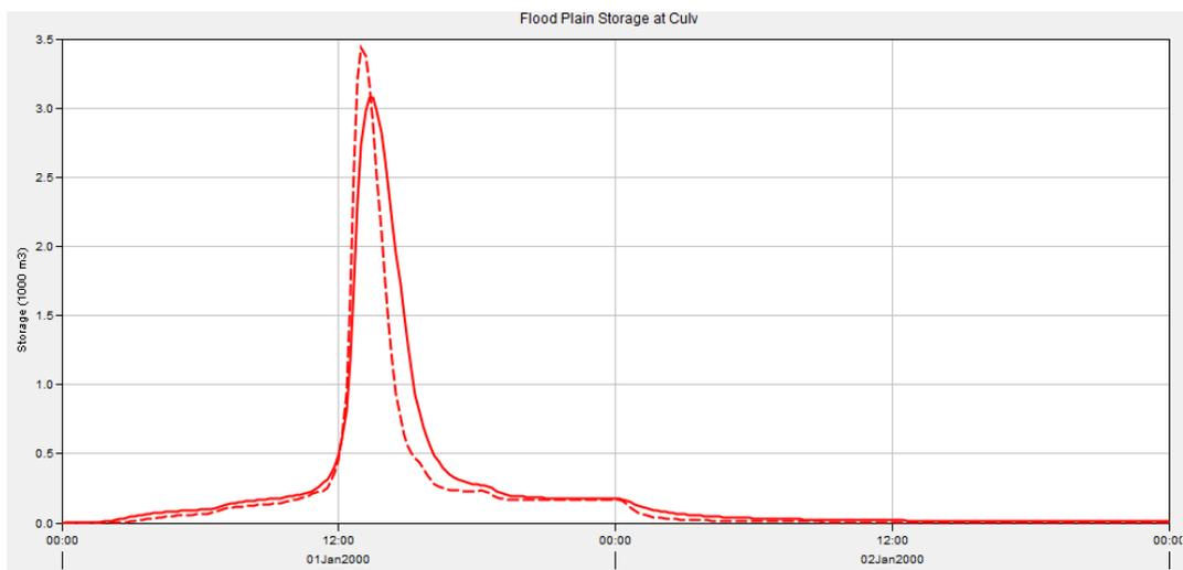
Figure 7: Storage within the southern sub-catchment floodplain upstream of the railway culvert. Dashed line = pre-development scenario and the solid line = post-development scenario.
