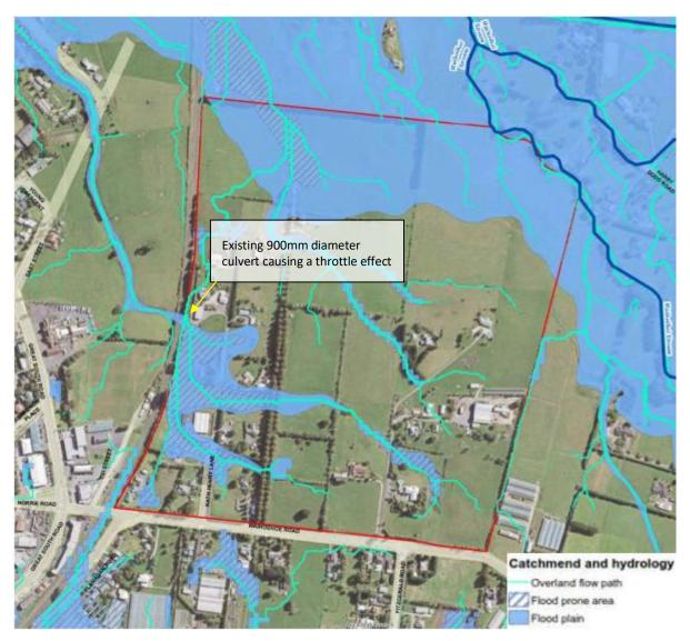
Figure 1: Flooding and overland flow paths within the Waihoehoe Precinct and railway culvert
