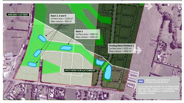
Figure 2: Indicative attenuation device locations within the southern sub-catchment of the Waihoehoe PCA
