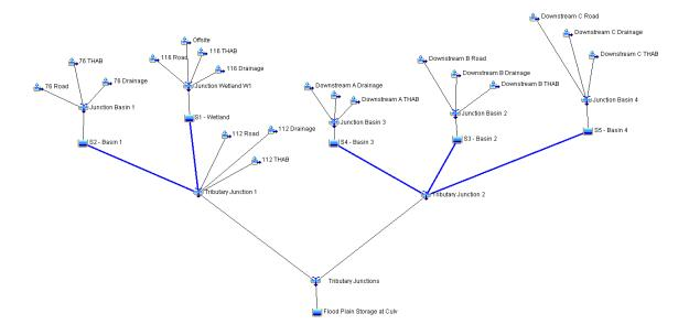
Figure 5: Post-development scenario basin model within HEC-HMS
