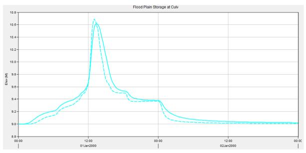
*Figure 8: Peak water levels within the southern sub-catchment floodplain upstream of the railway culvert. Dashed line = pre-development scenario and the solid line = post-development scenario.*
