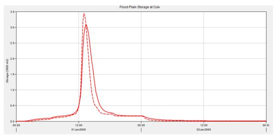
*Figure 7: Storage within the southern sub-catchment floodplain upstream of the railway culvert. Dashed line = pre-development scenario and the solid line = post-development scenario.*
