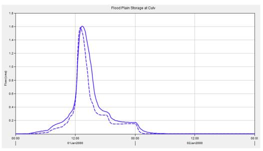
*Figure 6: Peak flowrates at the railway culvert within the Downstream sub-catchment. Dashed line = pre-development scenario and the solid line = post-development scenario.*
