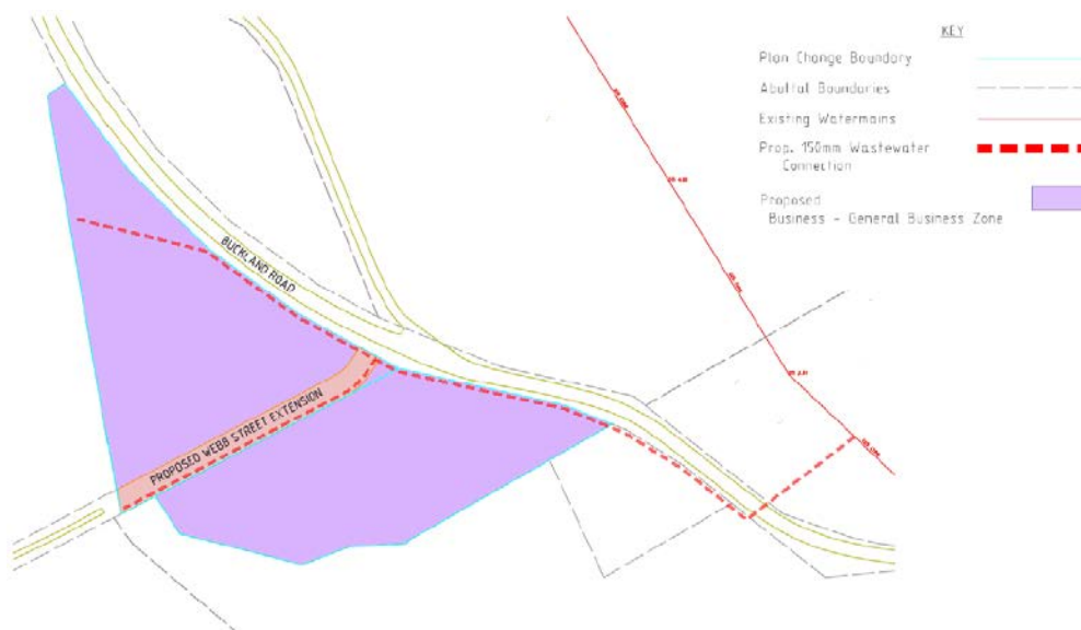
Figure 13: Proposed Wastewater Servicing for PC87
