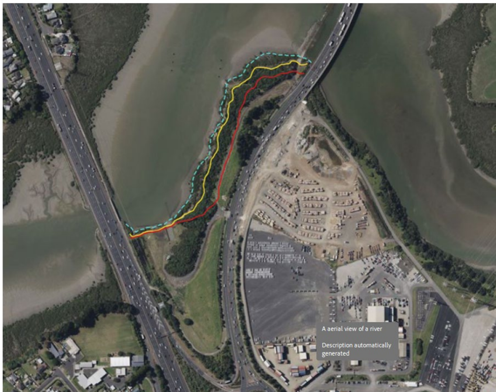
Figure 3: showing 100 year ASCIE line (red) calculated in eCoast Report. Yellow denotes shoreline and cyan denotes mangrove edge.
