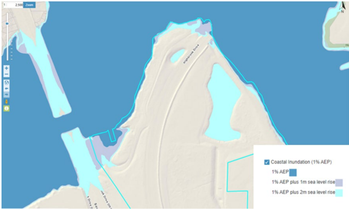
Figure 2.4 AC Geomaps Plan illustrating the Coastal Transition Zone and Coastal Inundation 1% AEP plus 1 m, and 2m SLR
