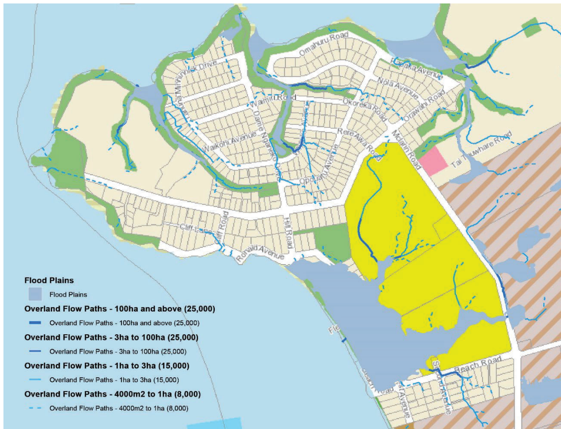
Figure 7: Flood plains and overland flow paths 145
