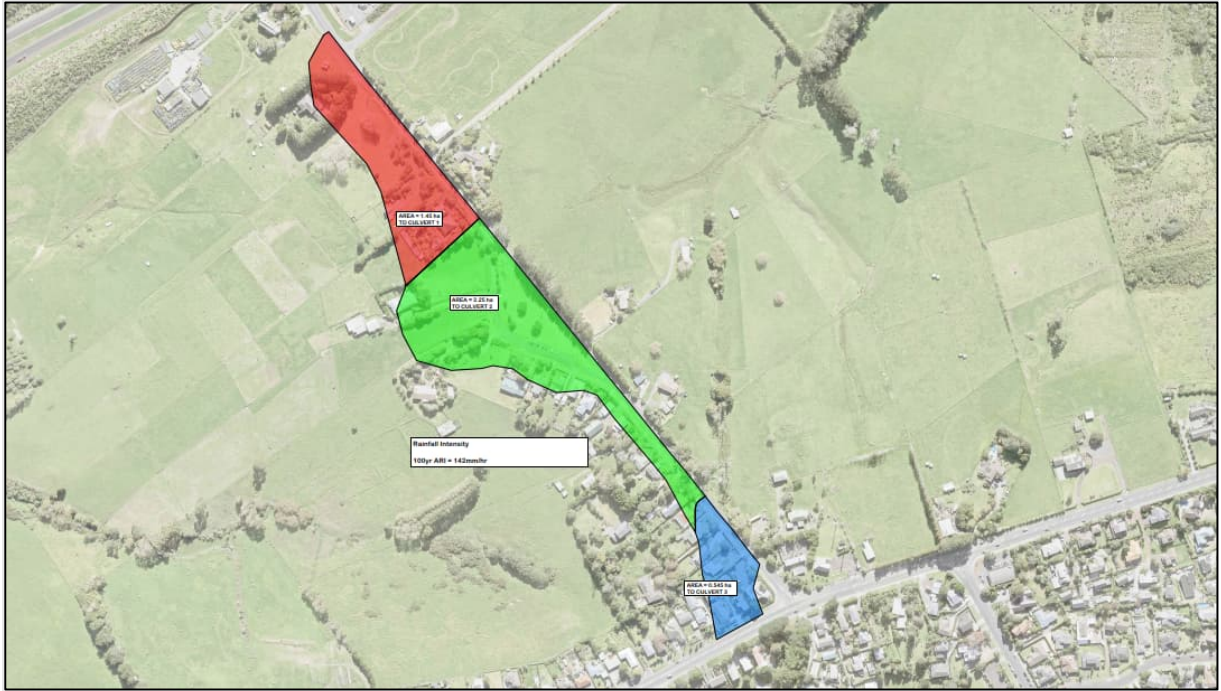
Figure 9: Pre-development catchments for culvert/pipe flows
