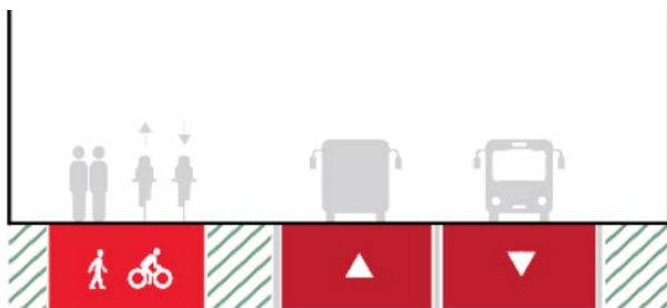
Figure 6-7: Typical Cross section – Rural Rapid Transit Corridor
