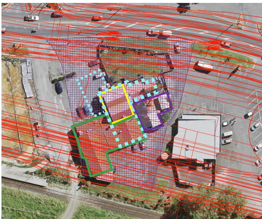
Yellow outline – surviving Pre-1900 Core; Blue outline – Pre-1940 footprint (approximate); Green outline– Pre1979; Purple - Pre-2006
