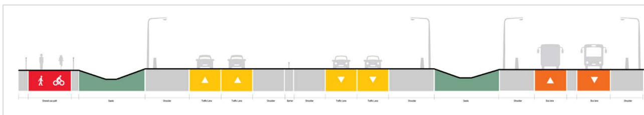
Figure 9-1: Rapid Transit Corridor Potential Cross-Sections
