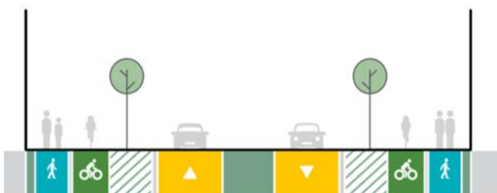
Figure 11-9: Coatesville-Riverhead Highway 24 m urban arterial
