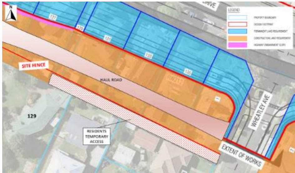
Figure 91: 129 Ti Rakau Dr temporary access
