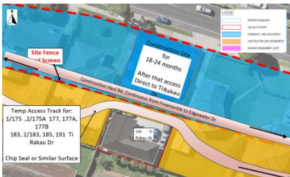
Figure 94: 191 Ti Rakau Dr temporary access
