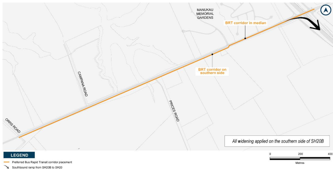
Figure 44: Preferred BRT placement and side of road widening option (SH20B)
