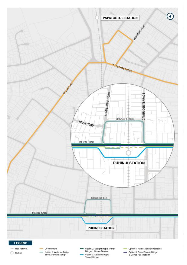
Figure 25: Puhinui Station Interchange Options, including Rapid Transit Bridge alignment
