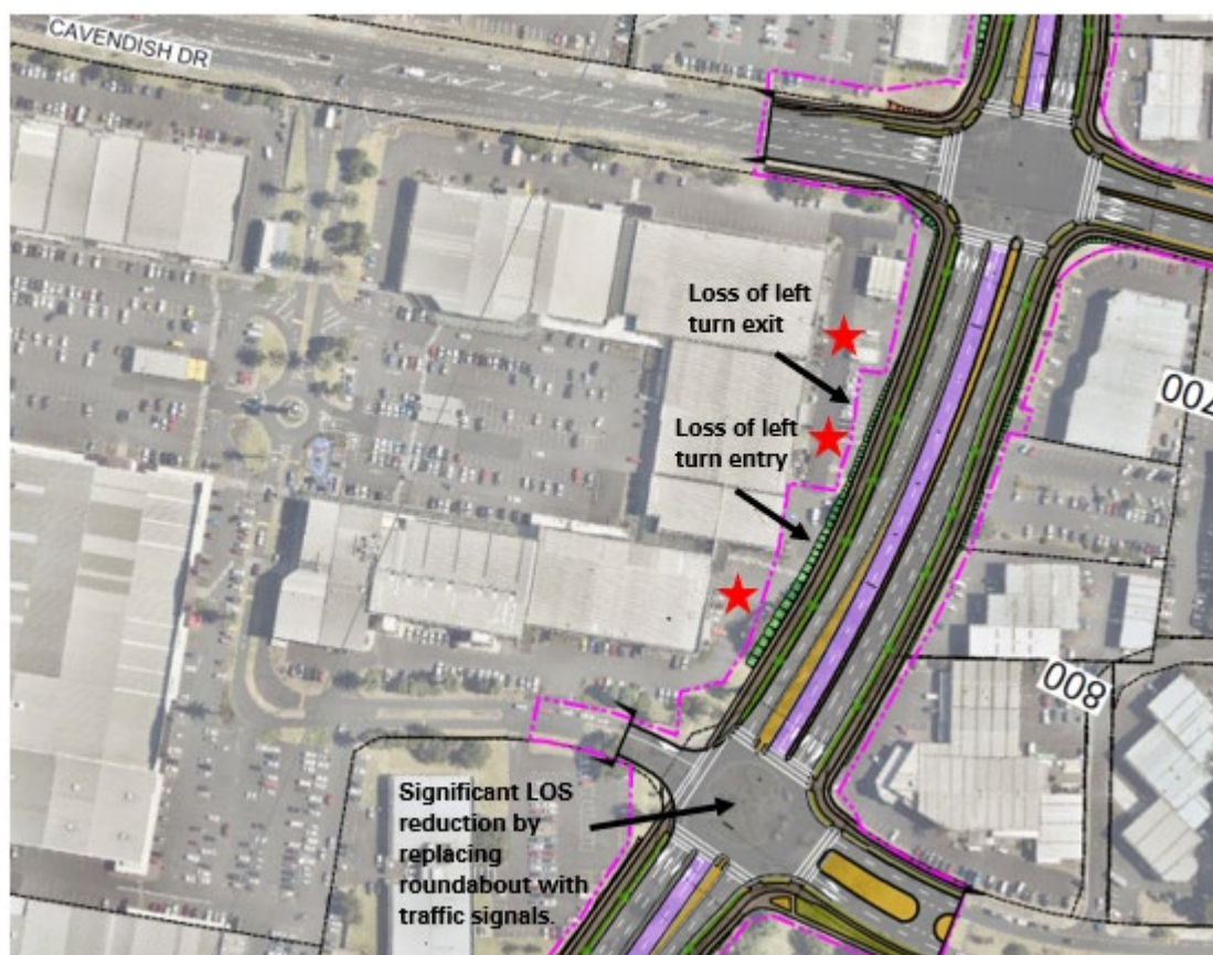
Figure 3: Portion of the 'General Arrangement Plan' as it relates to the Site. The pink dotted line refers to the proposed designation boundary. The green hatch is fill batter. Compromised truck loading areas are shown as red star.
