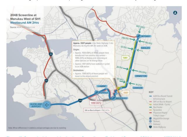
Figure 47: Demand origins and destinations. Screenline on Te Irirangi Dr, west of SH1 (source MSM i11.5 2048)
