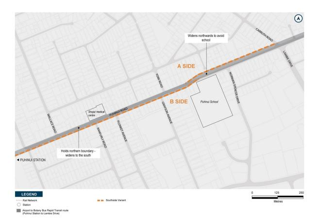
Figure 68: Southside variant option (initial preferred option was widening on the northern side entirely)
