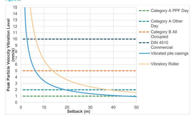
Figure 2: Vibration regression curves (criteria for occupied buildings)
