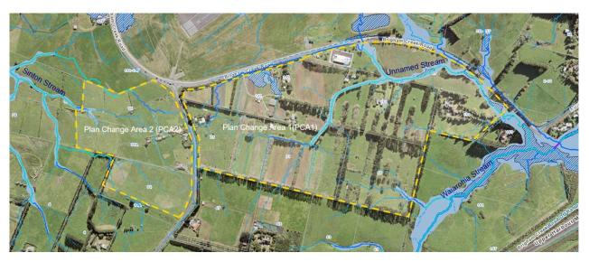
Figure 4. Diagram of area for PCA1 and PCA2, including box culvert (purple line) on Brigham Creek Road, overland flow paths, flood plains and flood prone areas from Auckland Council GeoMaps, source the proposed SMP, 22 October 2024
