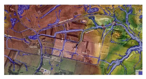
Figure 8. Post development flood extent from flood modelling with 3.8 degree climate change in a 1% AEP storm event , source the proposed SMP, 22 October 2024
