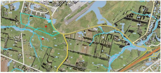
Figure 18. 131-137 and 139 Brigham Creek Road (red dots), the streams (Sinton Stream at the western side and the Waiarohia Stream at the eastern side of the diagram, box culvert (purple line), and flood plains in the surrounding environment, source Auckland Council GeoMaps, March 2025
