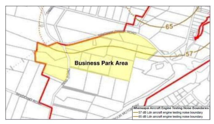
Figure 12 Engine Testing Noise Contours applying to PPC 107 (Source: The Acoustic Assessment supporting the Plan Change Request, Fig. 3)
