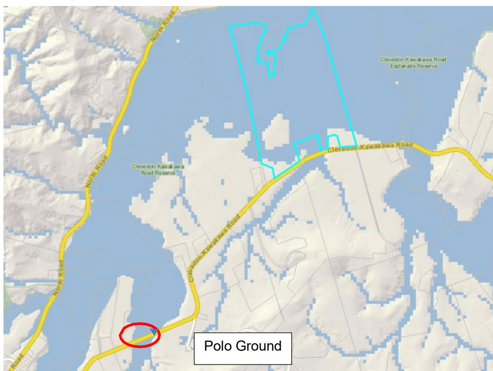
Figure 3: A view the 1% AEP floodplain around Polo ground area and the PC45 site
