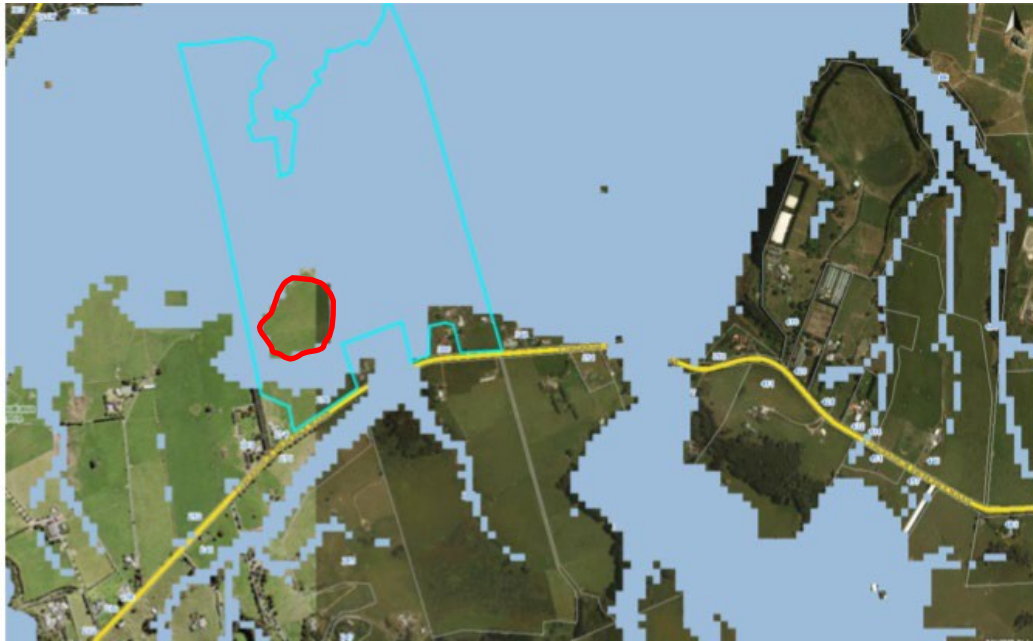
Figure 1: Extent of the 1% AEP flood plain in the surrounding area (Red area indicates the land outside 1% AEP floodplain)
