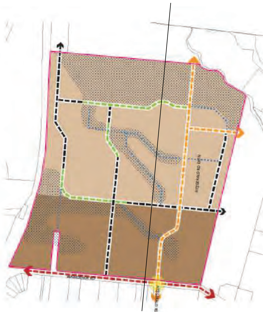
Figure 10 Proposed Structure Plan — Plan Change Area Boundary ■ Southern SW sub-catchment coverage control area ■ Northern SW sub-catchment coverage control area ■ Collector Road ■ Local Road ■ Park Edge Road ● Signalled Intersection □ Drainage Reserve (to be defined through detail design) ● Existing Wetlands ●●● Green Link / Swale ▨ Potential Waiohohoe Rd widening. Depth and dimension to be confirmed at a later
