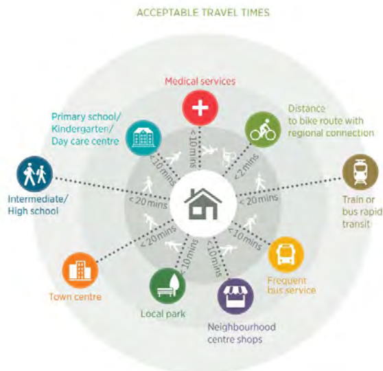
Figure 37: Acceptable travel times (extract from AT's Urban Streets and Road Design Guide)
