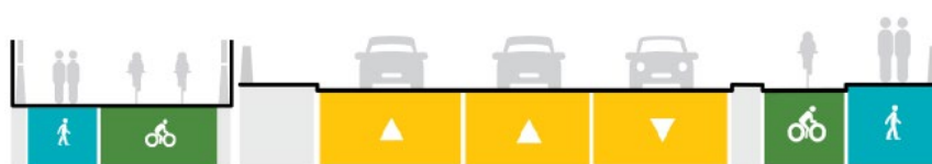
Figure 10-7: NOR W1: Trig Road (North) typical cross section – existing bridge and new active mode bridge
