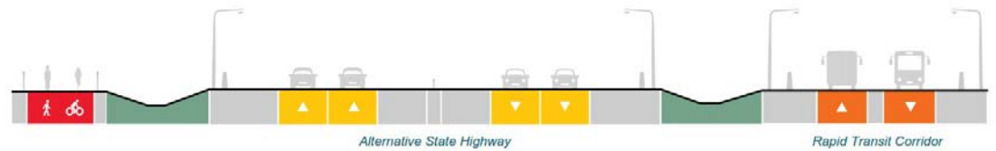
Figure 10-17: Typical Cross Section – RTC alongside ASH at Taupaki Road (shared path will re-join RTC at Boord Crescent)
