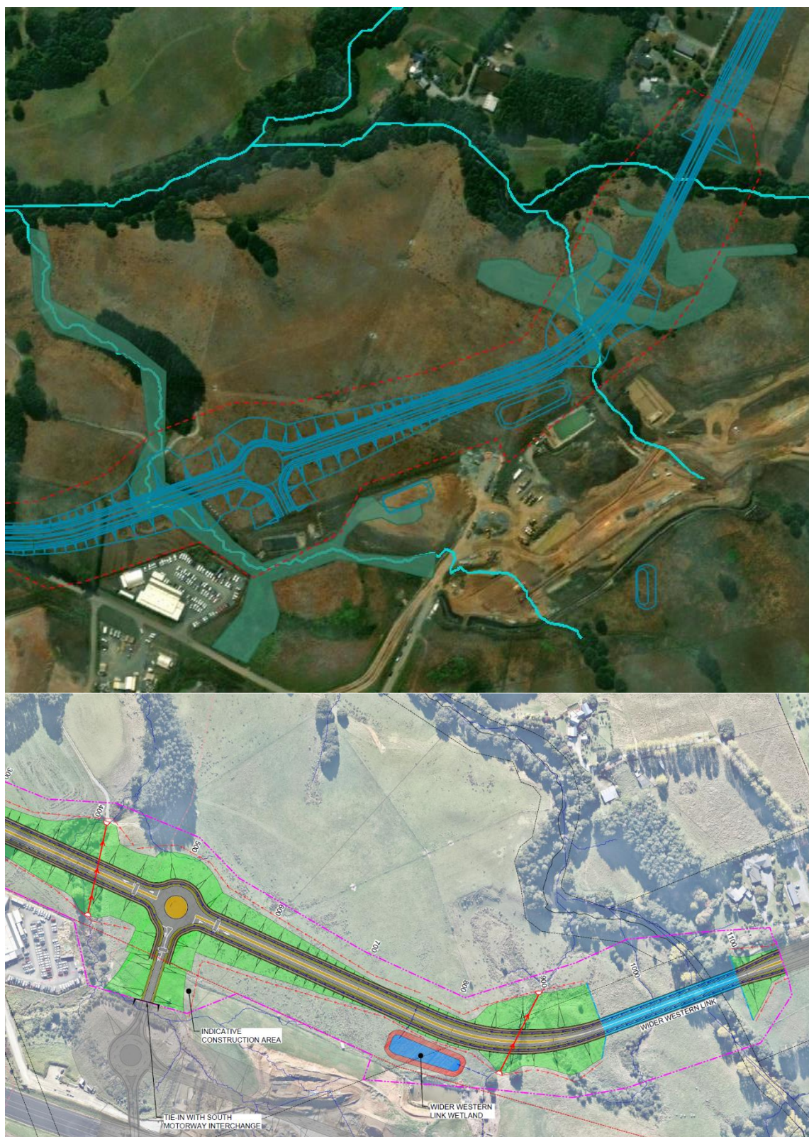
Figure 17-1 Natural wetlands are indicated by areas of green in the top image. Areas of fill are shown in bright green in the bottom image.
