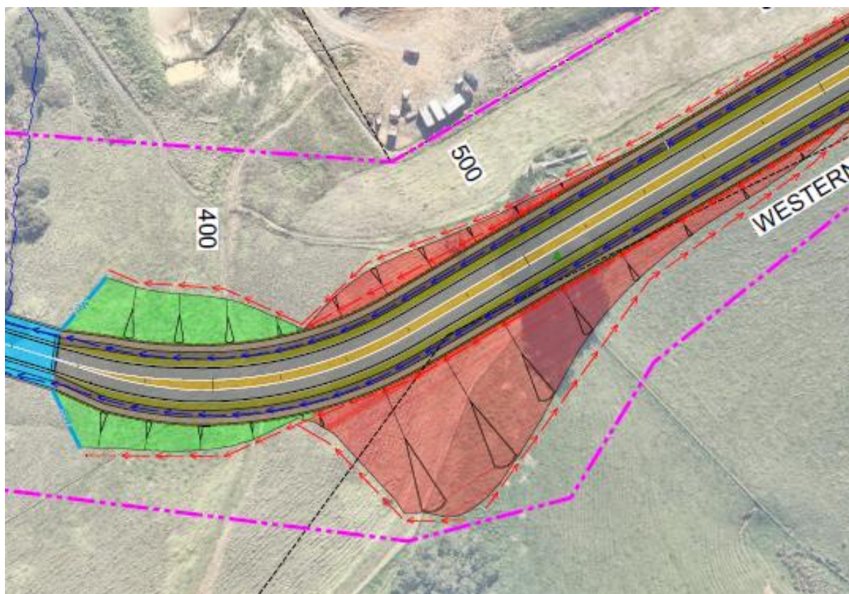
Figure 15-2 Minimal space between large cut area and designation boundary could potentially result in benched cuts.
