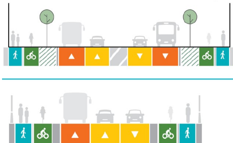
Figure 6: typical four-lane and three-lane FTN arterial cross sections applied to sections of the Great South Road FTN
