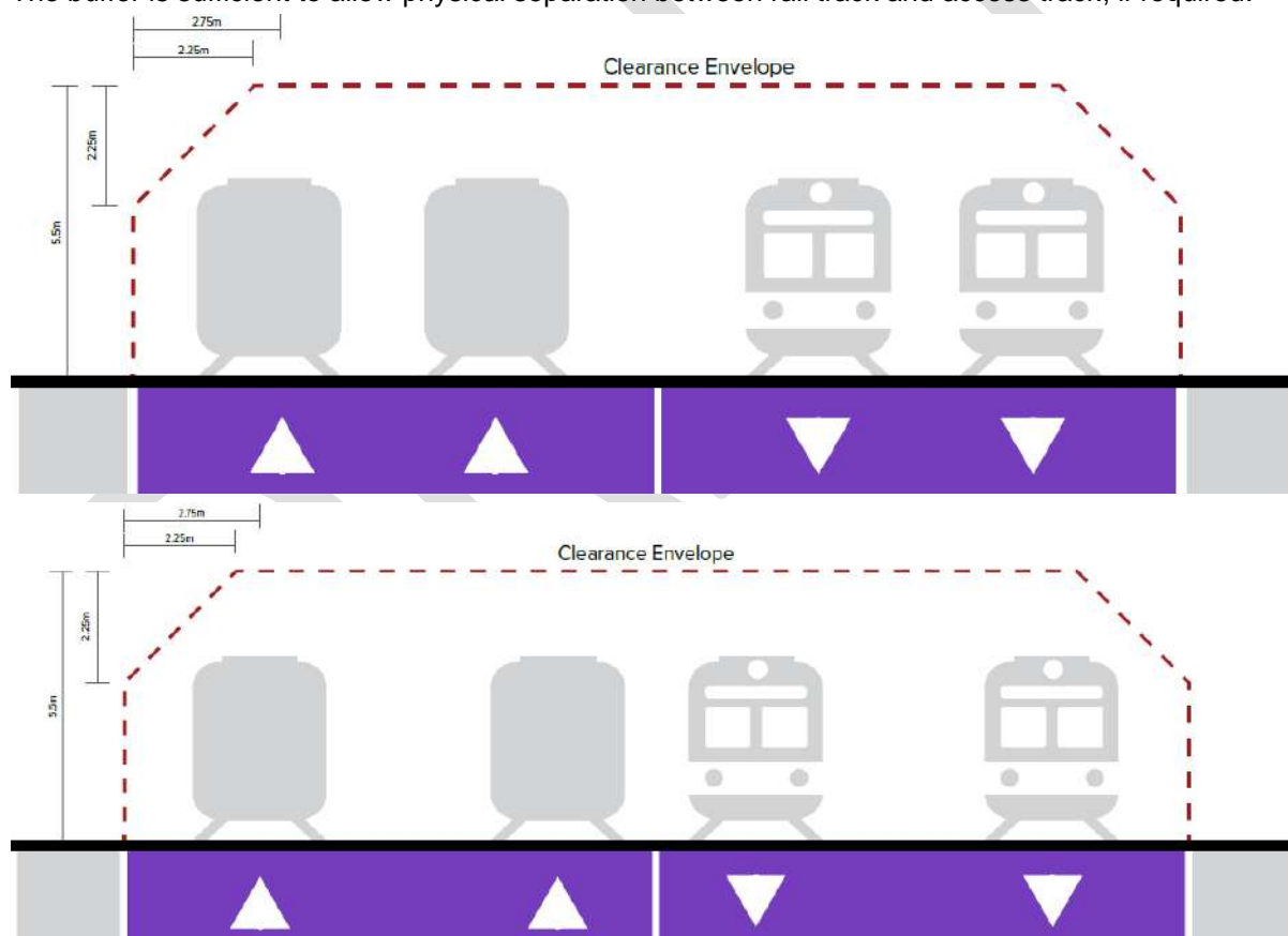
Figure 2-2 General clearance requirements for four-tracking, with two future tracks to one side of existing tracks (top) and a future track to either side of existing tracks (bottom).
