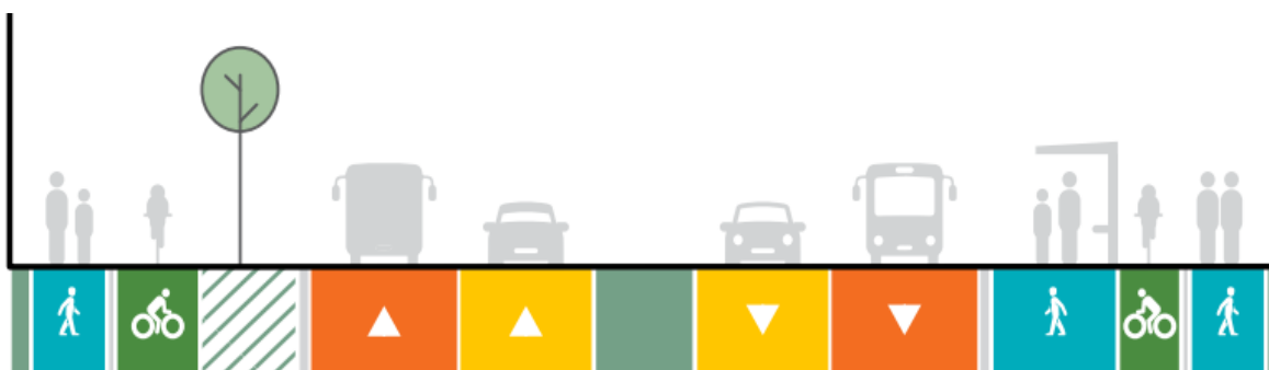
Figure 4-2: Four-lane FTN arterial cross-section
