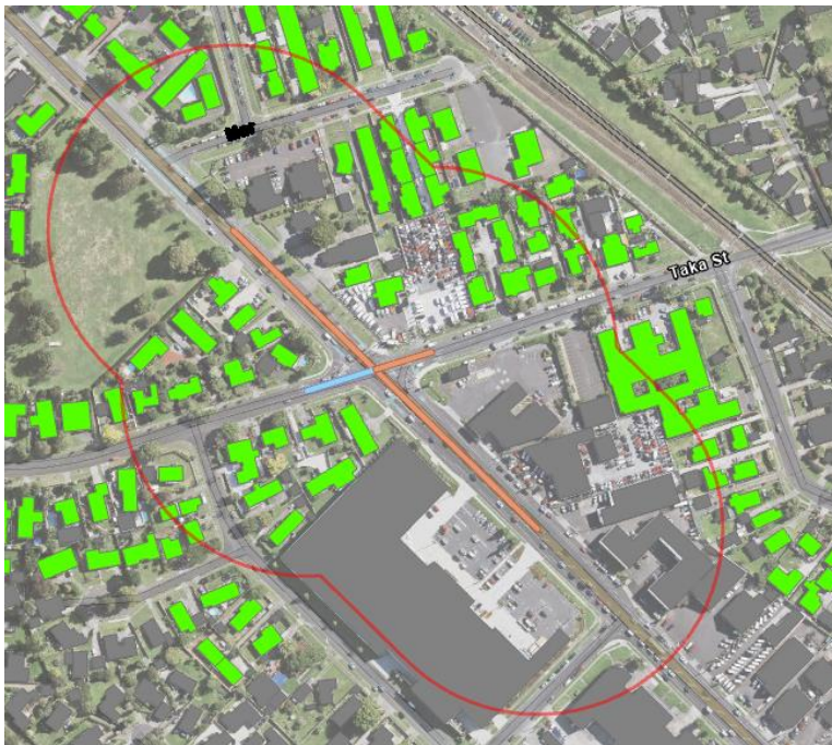
Figure 7-5: NoR 1-D – extent and road surface finishes (orange – AC-14, blue – chipseal)
