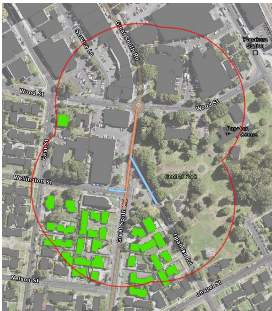
Figure 7-9: NOR 1-F – extent and road surface finishes (orange – AC-14, blue – chipseal)
