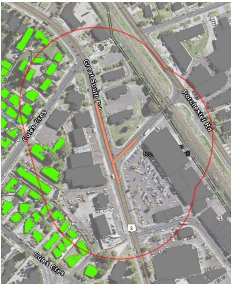
Figure 7-7: NOR 1-E – extent and road surface finishes (orange – AC-14)
