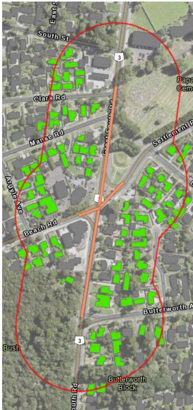
Figure 7-11: NoR 1-G – extent and road surface finishes (orange – AC-14)
