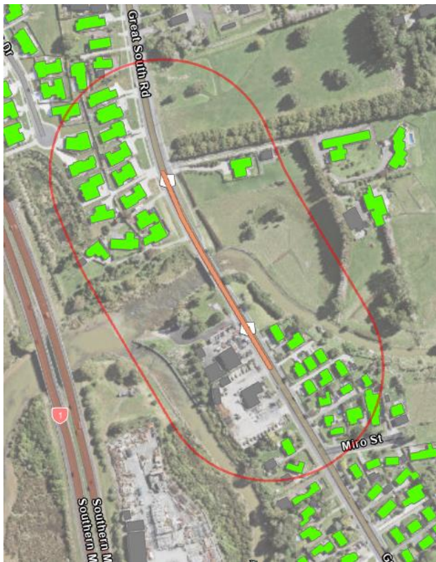
Figure 7-15: NOR 1-Bridge – extent and road surface finishes (orange – AC-14)
