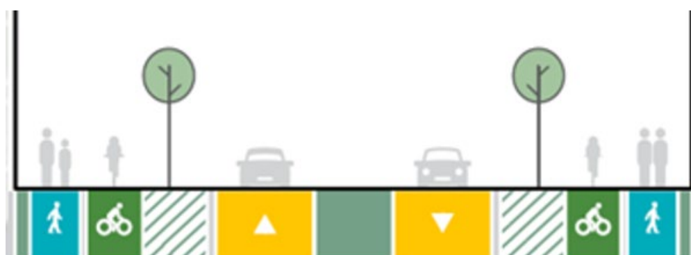
Figure 5-11: Two-lane FTN arterial as proposed for section 7-9 of the Takaanini FTN
