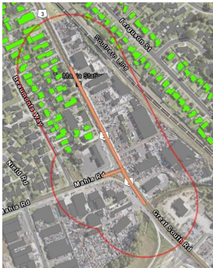
Figure 7-3: NoR 1-C – extent and road surface finishes (orange – AC-14)
