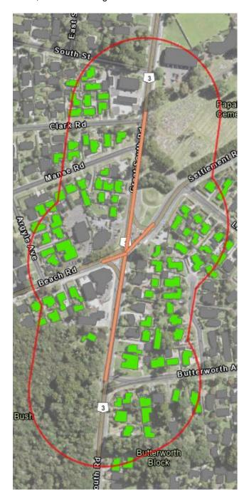
Figure 7-11: NoR 1-G – extent and road surface finishes (orange – AC-14)
