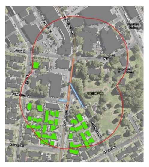
Figure 7-9: NOR 1-F – extent and road surface finishes (orange – AC-14, blue – chipseal)
