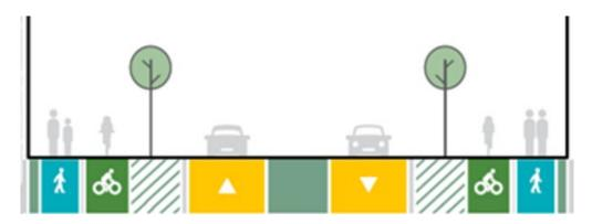
Figure 5-11: Two-lane FTN arterial as proposed for section 7-9 of the Takaanini FTN
