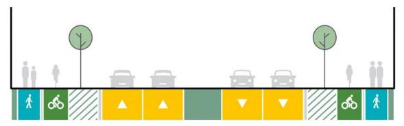
Figure 6-3: Four-lane arterial as proposed for Great South Road (Drury).
