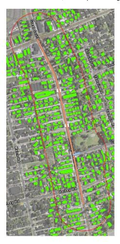
Figure 7-1: NoR 1-A-B - extent and road surface finishes (orange - AC-14, blue - chipseal)
