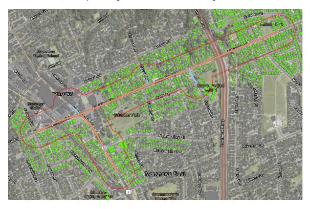
Figure 9-1: NOR 3 – extent and road surface finishes (orange – AC-14, blue – chipseal)
