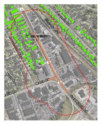
Figure 7-3: NoR 1-C – extent and road surface finishes (orange – AC-14)
