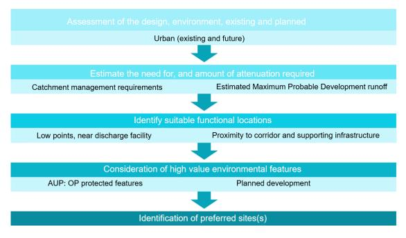
Figure 3-2: Stormwater infrastructure design and location approach
