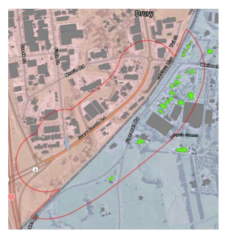
Figure 8-1: Road surface finishes (orange - AC-14, blue - chipseal), and urban (orange) and rural (light
