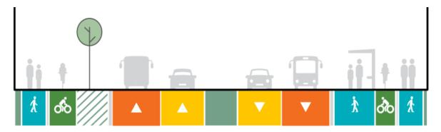
Figure 4-2: Four-lane FTN arterial cross-section
