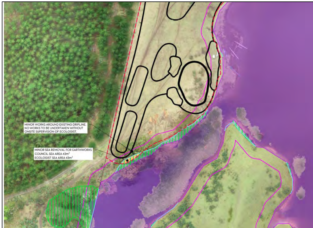
Figure 78: Extent of ONF boundary in green hatch. Area Affected by Earthworks Denoted by Orange Area)
