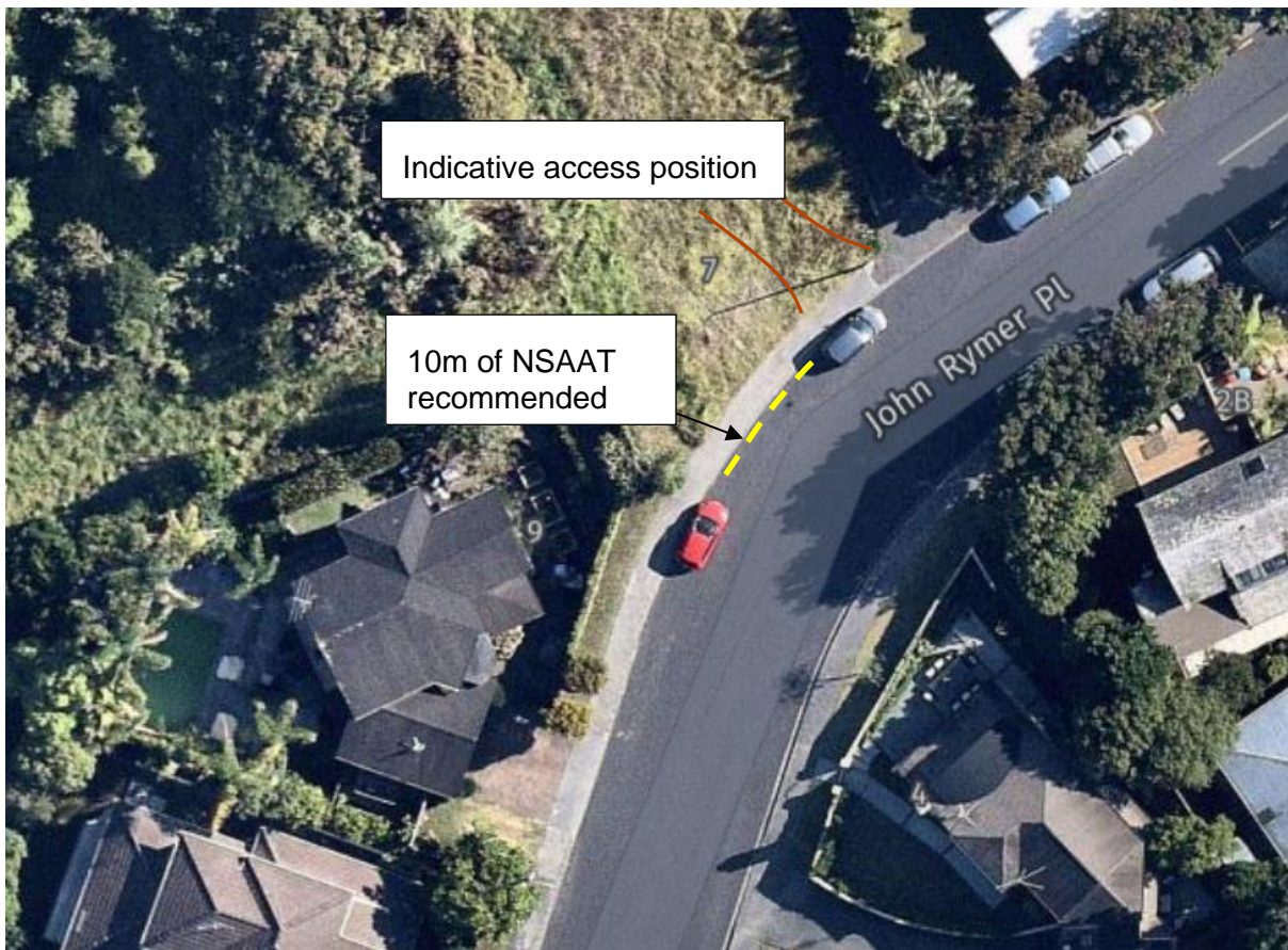
Figure 5-7: No stopping at all times markings recommended
