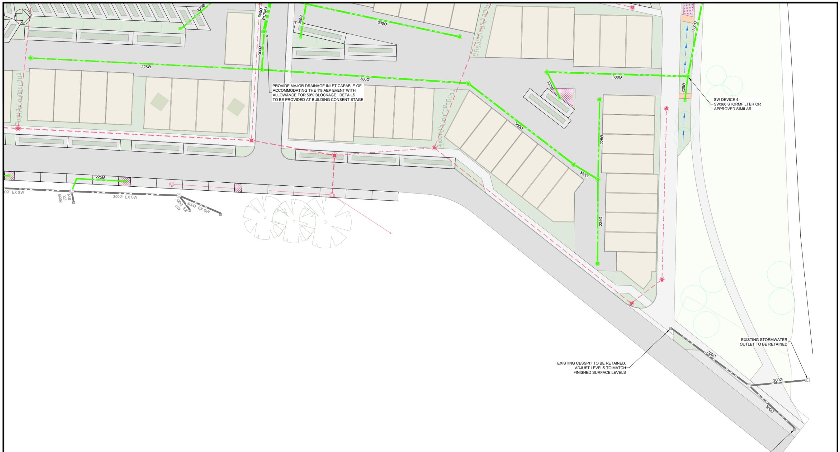
PROVIDE MAJOR DRAINAGE INLET CAPABLE OF ACCOMMODATING THE 1% AEP EVENT WITH ALLOWANCE FOR 50% BLOCKAGE. DETAILS TO BE PROVIDED AT BUILDING CONSENT STAGE
