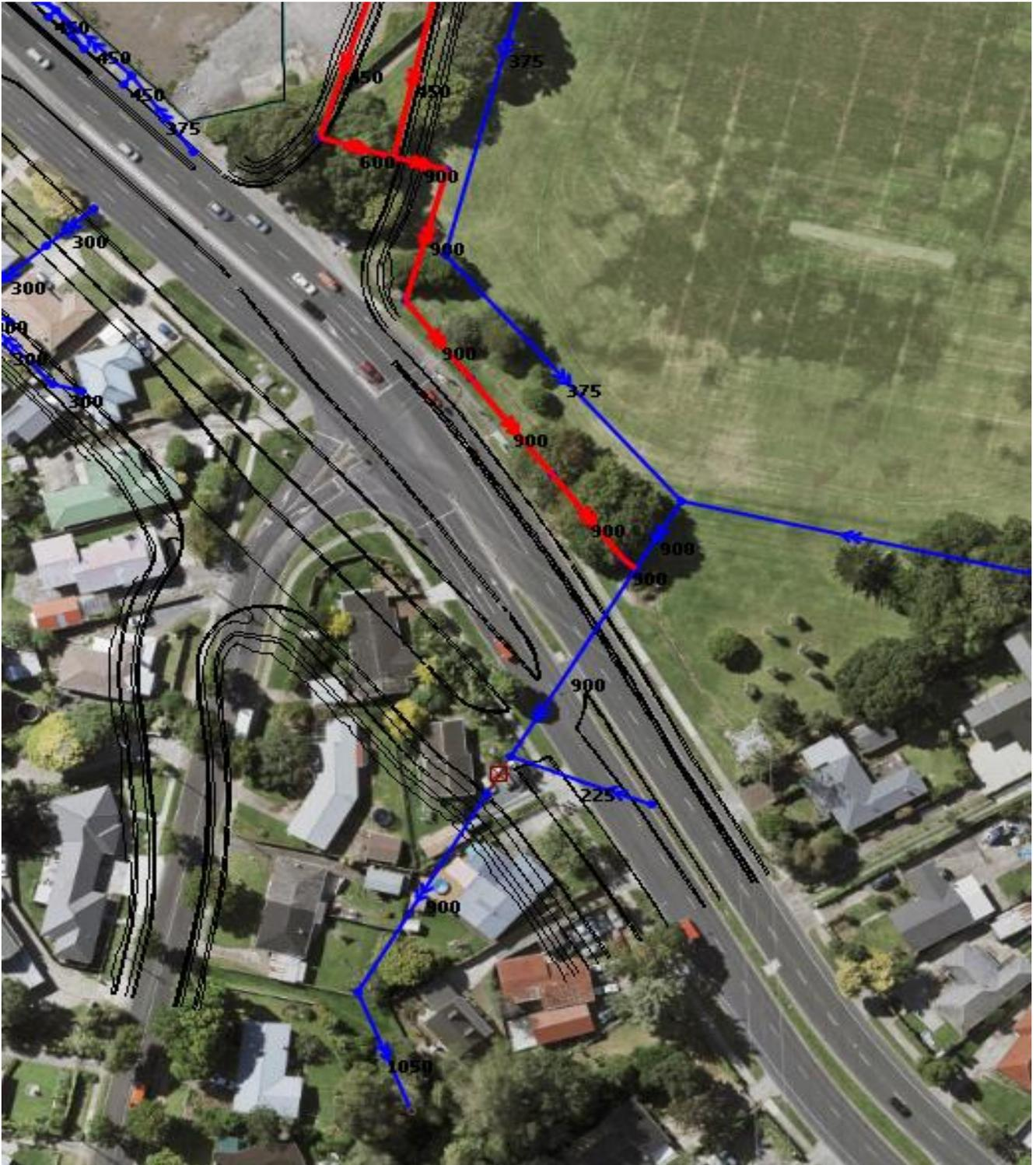
Figure 12: WRR design network highlighted in red connecting to the existing pipe network shown in blue.
