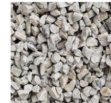
R.01 - Sandstone Chip Membrane roof with chip over.
