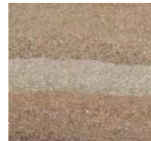
W.02 - Rammed Earth Rammed earth with local sandstone.
