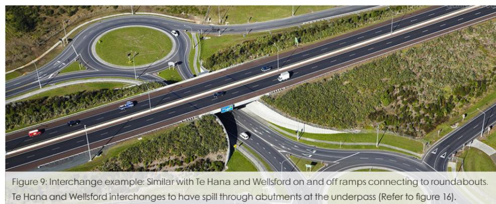
Figure 9: Interchange example: Similar with Te Hana and Wellsford on and off ramps connecting to roundabouts. Te Hana and Wellsford interchanges to have spill through abutments at the underpass (Refer to figure 16).
