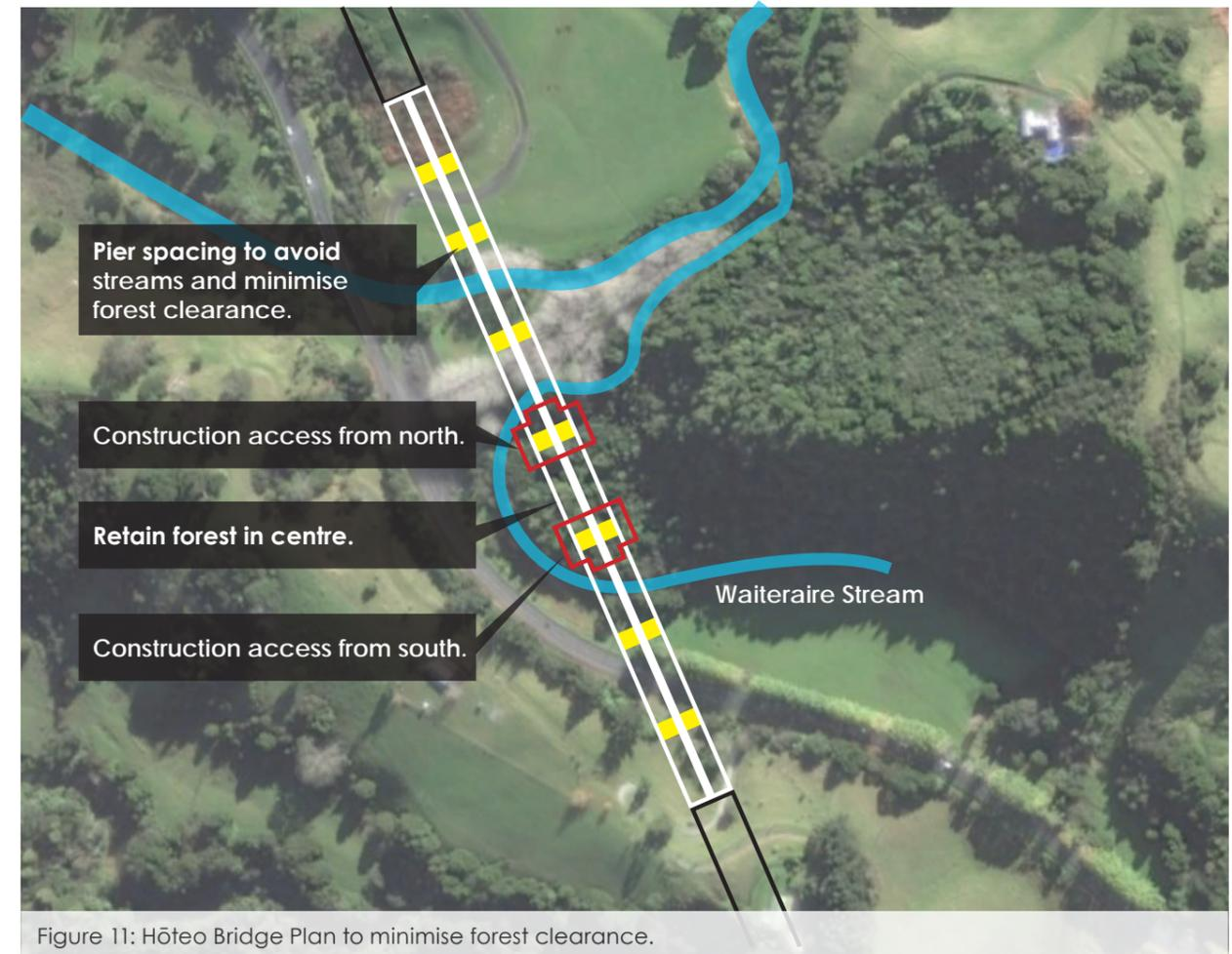
Figure 11: Hōteio Bridge Plan to minimise forest clearance.
