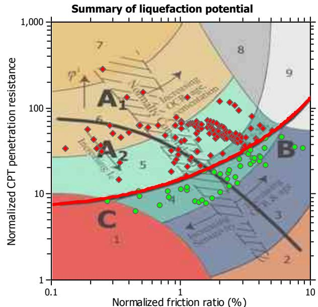
Zone A<sub>1</sub>: Liquefaction likely depending on size and duration of cyclic loading
