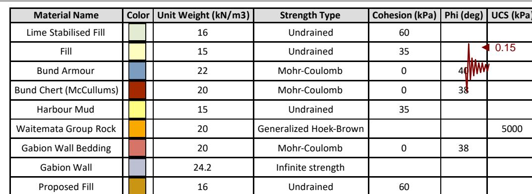
Run 10 - Seismic (NZGS Guidance Module 1),
