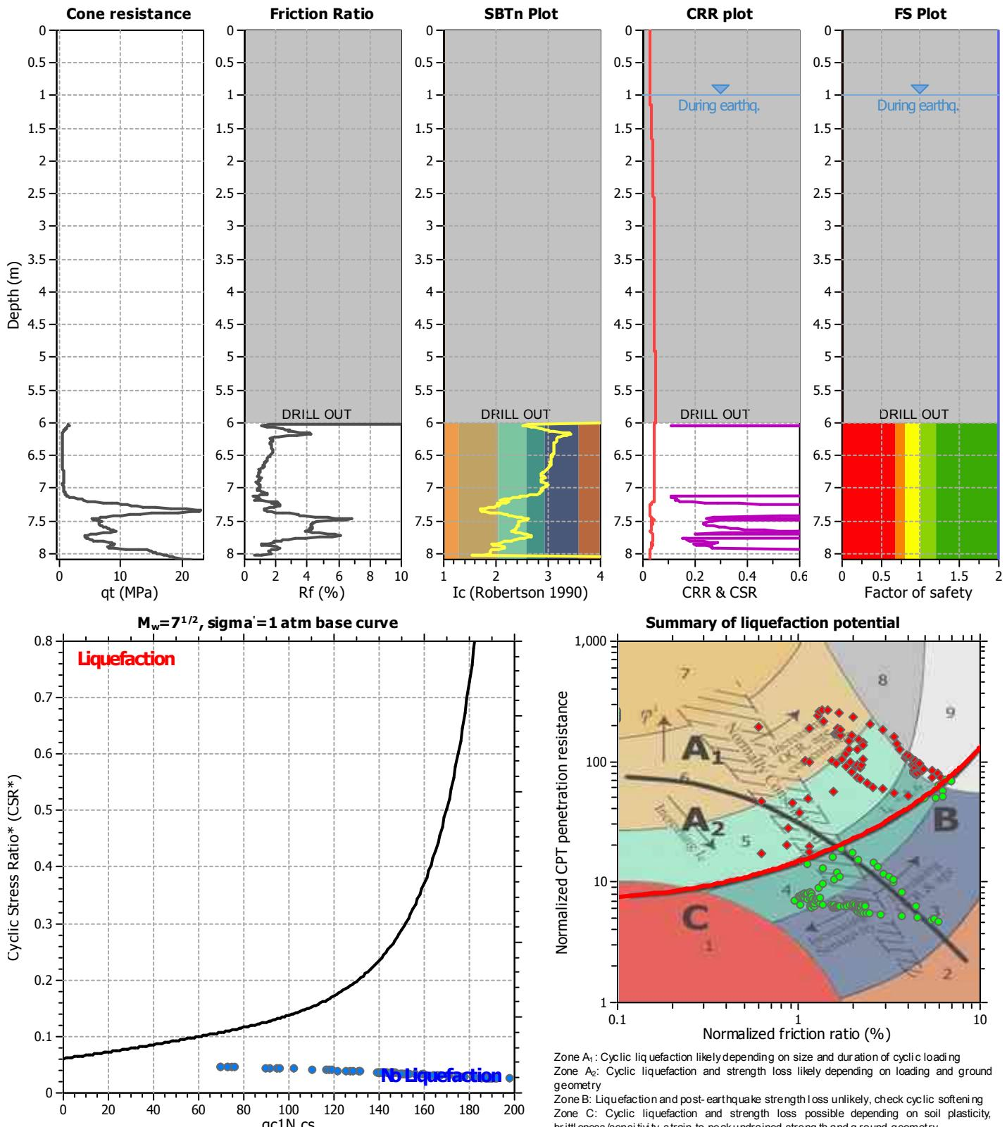
Zone A<sub>1</sub>: Cyclic liquefaction likely depending on size and duration of cyclic loading
