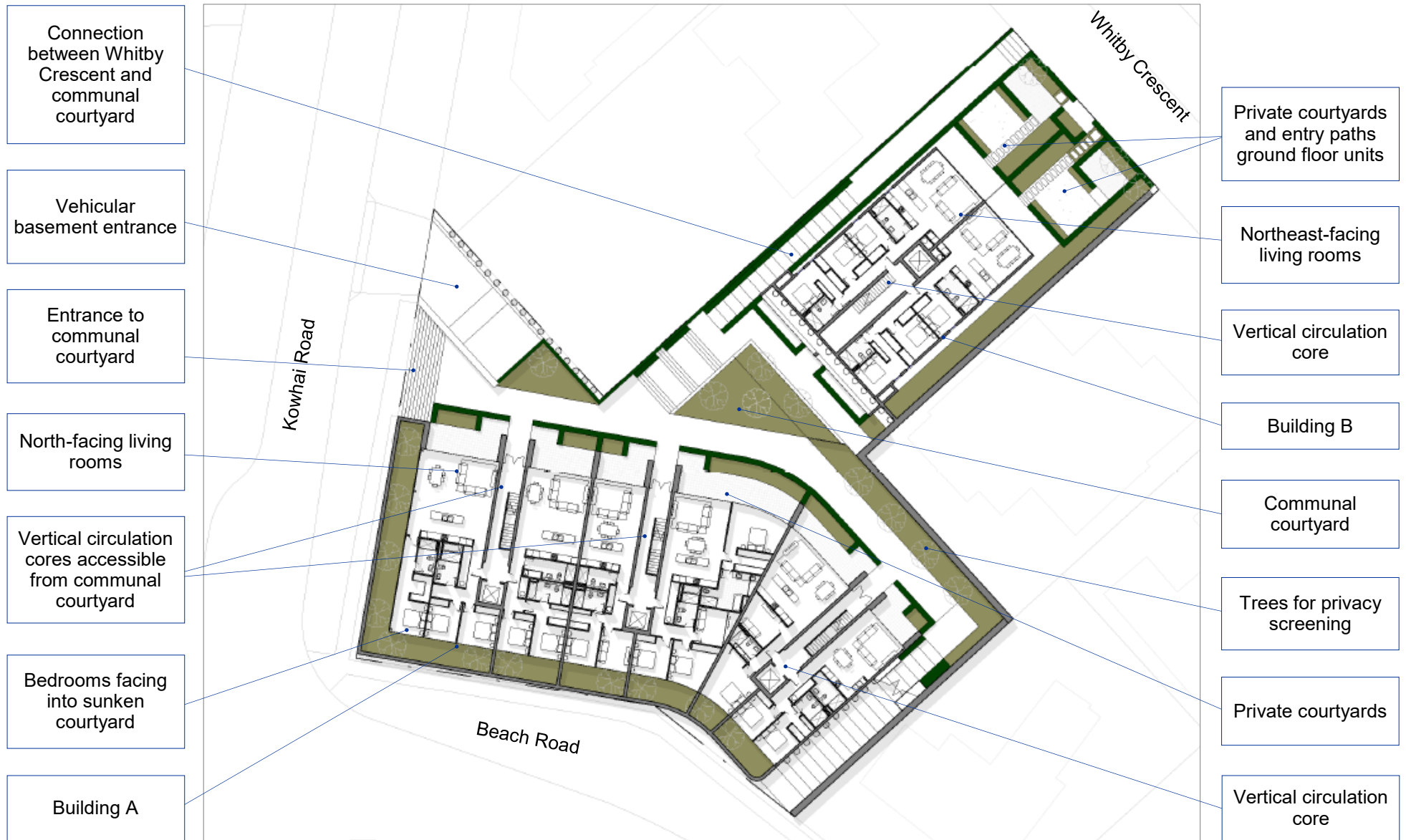
ABOVE FIG. 3-2: Proposed design key attributes Level 1 (Whitby Crescent street level and courtyard level).
