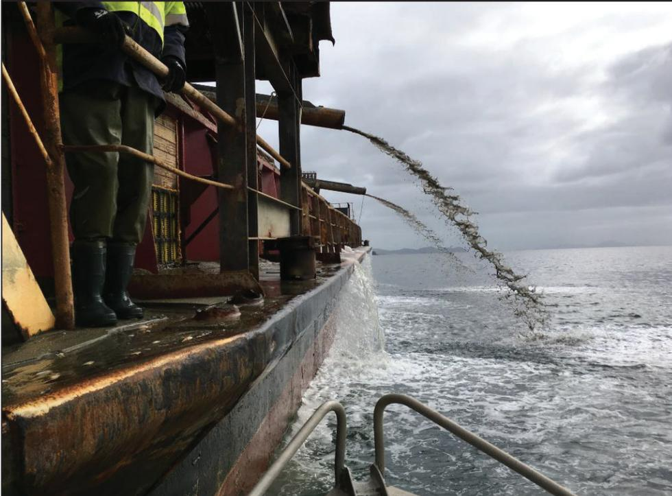
Figure 2-3: Discharge from the Coastal Carrier of by-wash from overhead flumes and from the deck over hopper weir boards.
