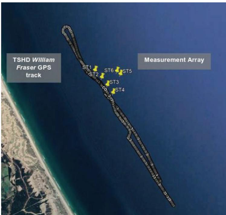
Figure 4-16: PS track of the TSHD William Fraser in relation to the measurement (hydrophone) array (ST1 through 6) on 28 November 2019 in fine weather conditions. (Source: Styles Group)
