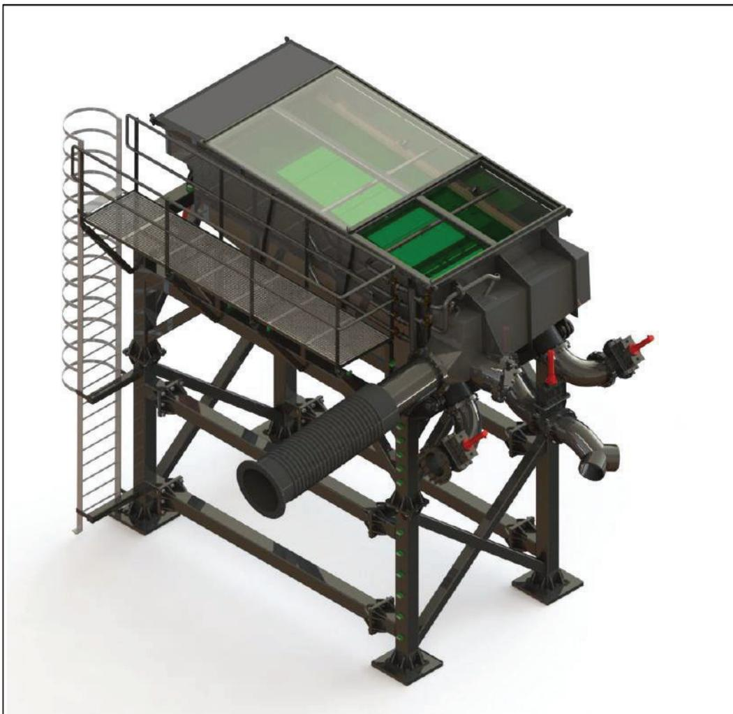
Figure 2-4: Diagram of sand “Screening Deck” on the ‘William Fraser’
