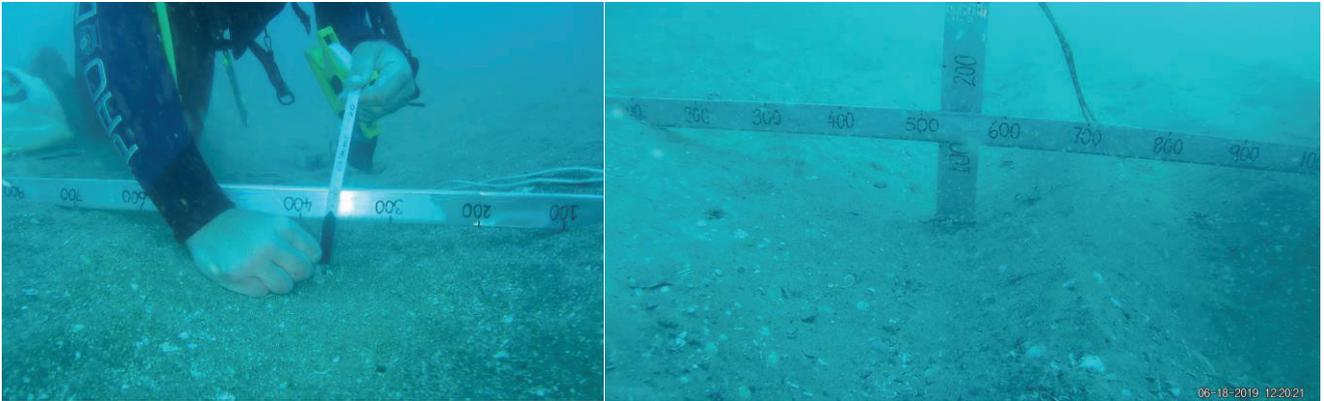
Figure 2.2: Dredge trench infill measurement methodology
