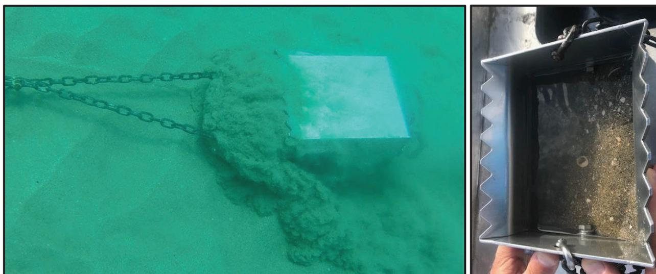
**Figure 2.1** Box dredge in operation and full retrieved sample
