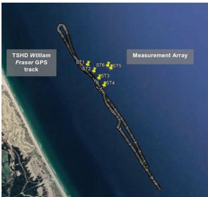
Figure 4-15: PS track of the TSHD William Fraser in relation to the measurement (hydrophone) array (ST1 through 6) (Source: Styles Group)
