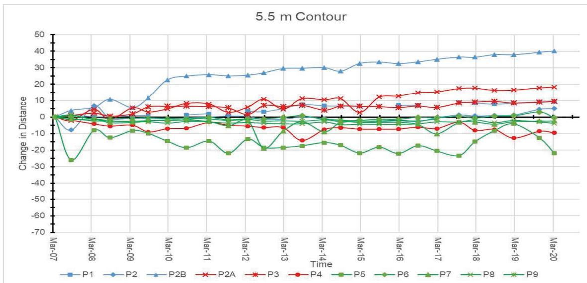
Figure 3.19: Excursion Distance plot of the 5.5m contour (proxy of dune face position) at historic profile sites 2007 – 2020.
