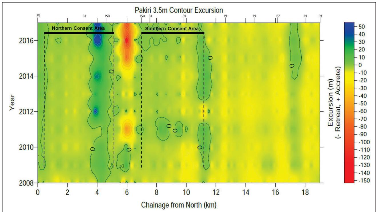
Figure 3.20: Three dimensional temporal-spatial map of distance excursion of the 3.5 m contour from topographic surveys 2007-2017
