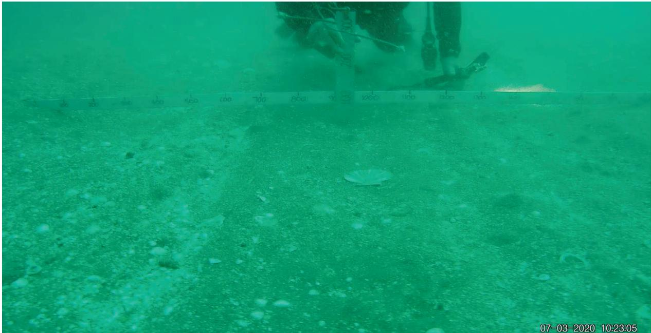
Figure 4.1: Imprint of 'William Fraser dredge trench' in 27.8 m CD water depth 36 hours post dredging.
