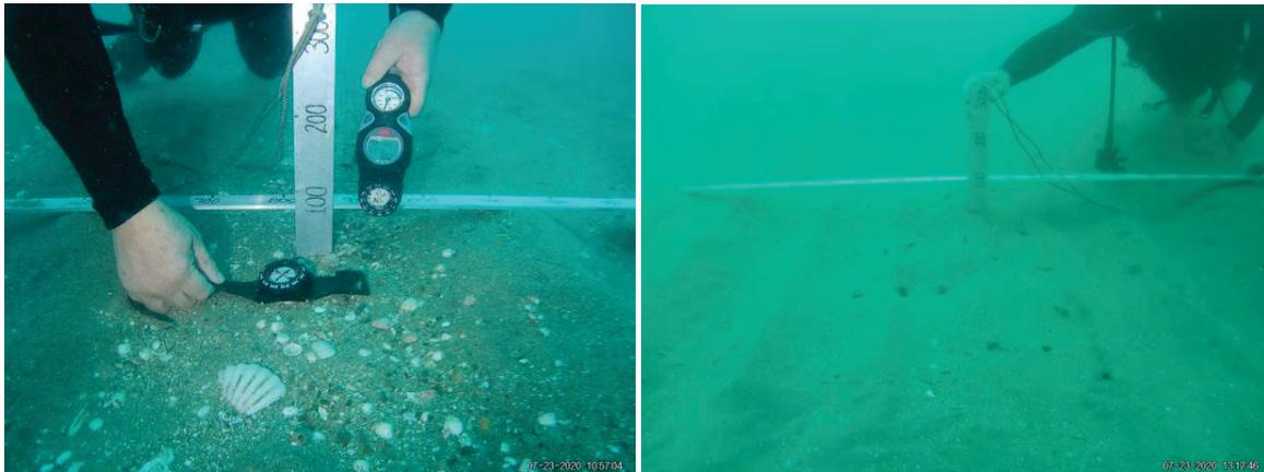
Figure 2.2: Dredge trench infill measurement methodology. Photos from William Fraser trenches.
