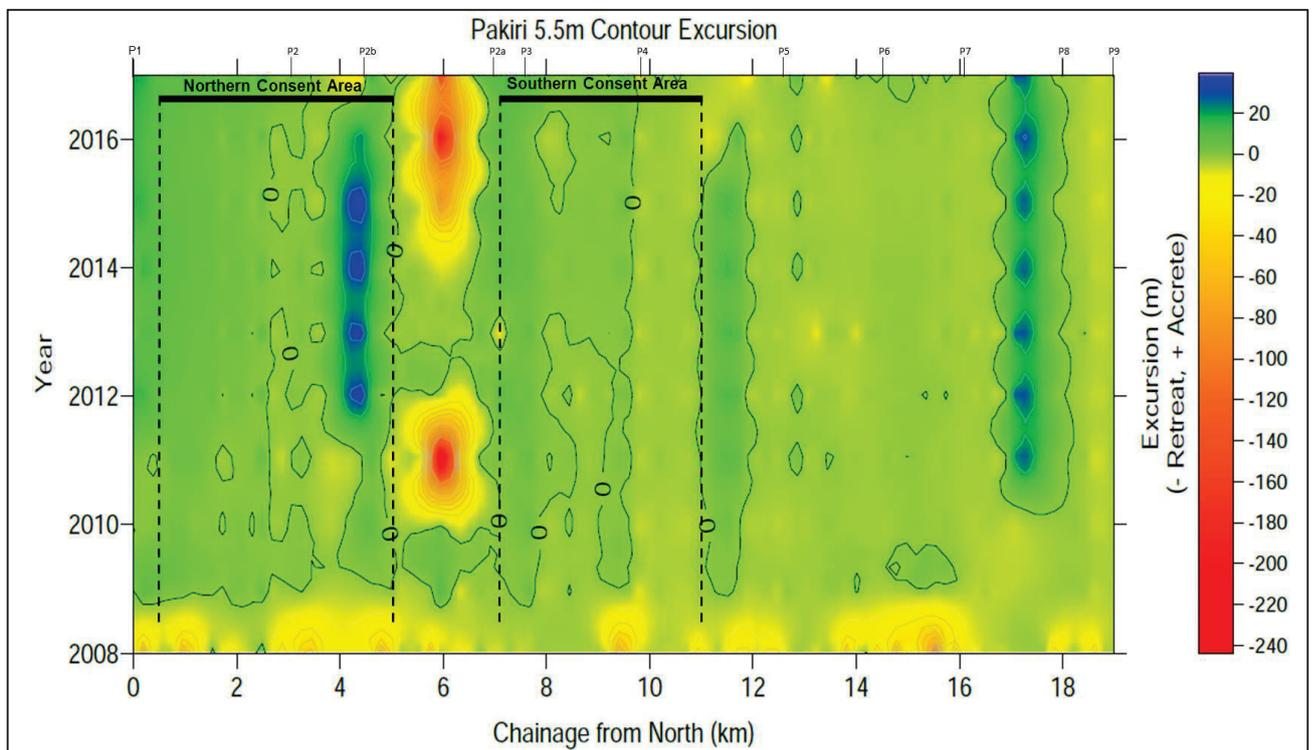
Figure 3.21: Three dimensional temporal-spatial map of distance excursion of the 5.5 m contour from topographic surveys 2007-2017
