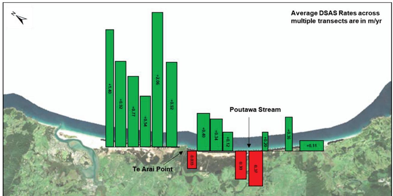
Figure 3.17: Spatial distribution of total shoreline change 1961/63 to 2018 from aerial photographs or from long-term beach profiles P5 & P6 since 1978 south of Poutawa Stream where 1960's aerial photographs were not available.
