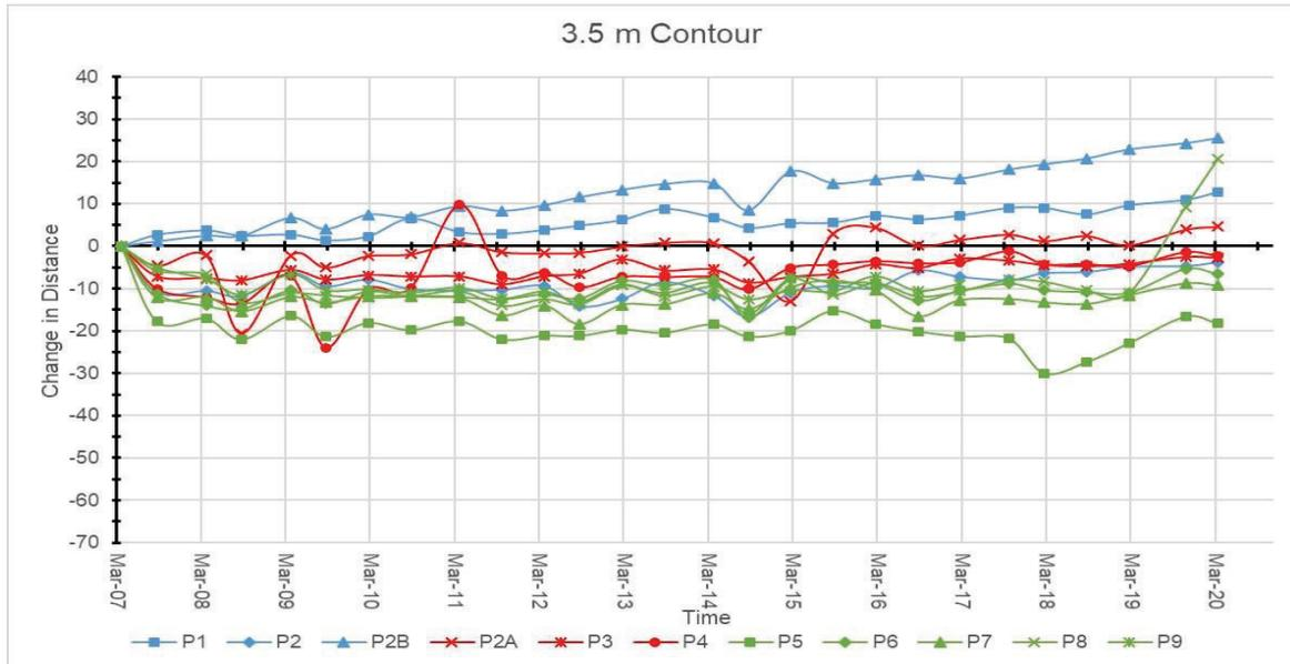
Figure 3.18: Excursion distance plot of the 3.5m contour (proxy for beach toe position) at historic profile sites 2007 – 2020
