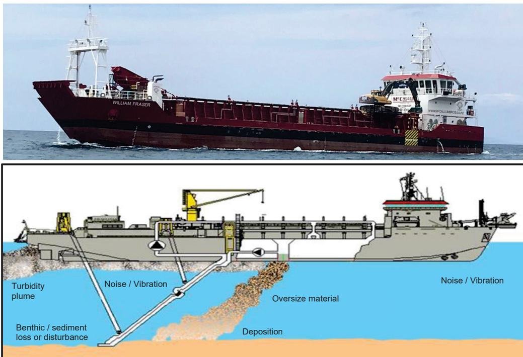
Figure 2. Top: MBL vessel, *William Fraser*, extracting sand from the current Pakiri coastal area. Bottom: Generic illustration of sand extraction and possible impacts, not all of which will be applicable to the current proposal (modified from Bioresearches 2019).
