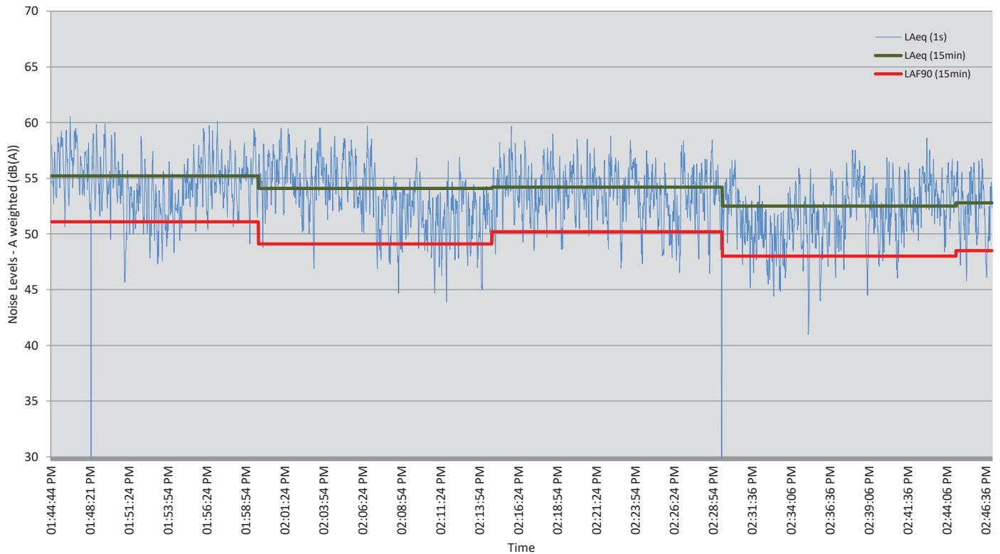
Pakiri Sand Extraction - Noise Level Measured at Position 5 - 22<sup>nd</sup> May 2019
