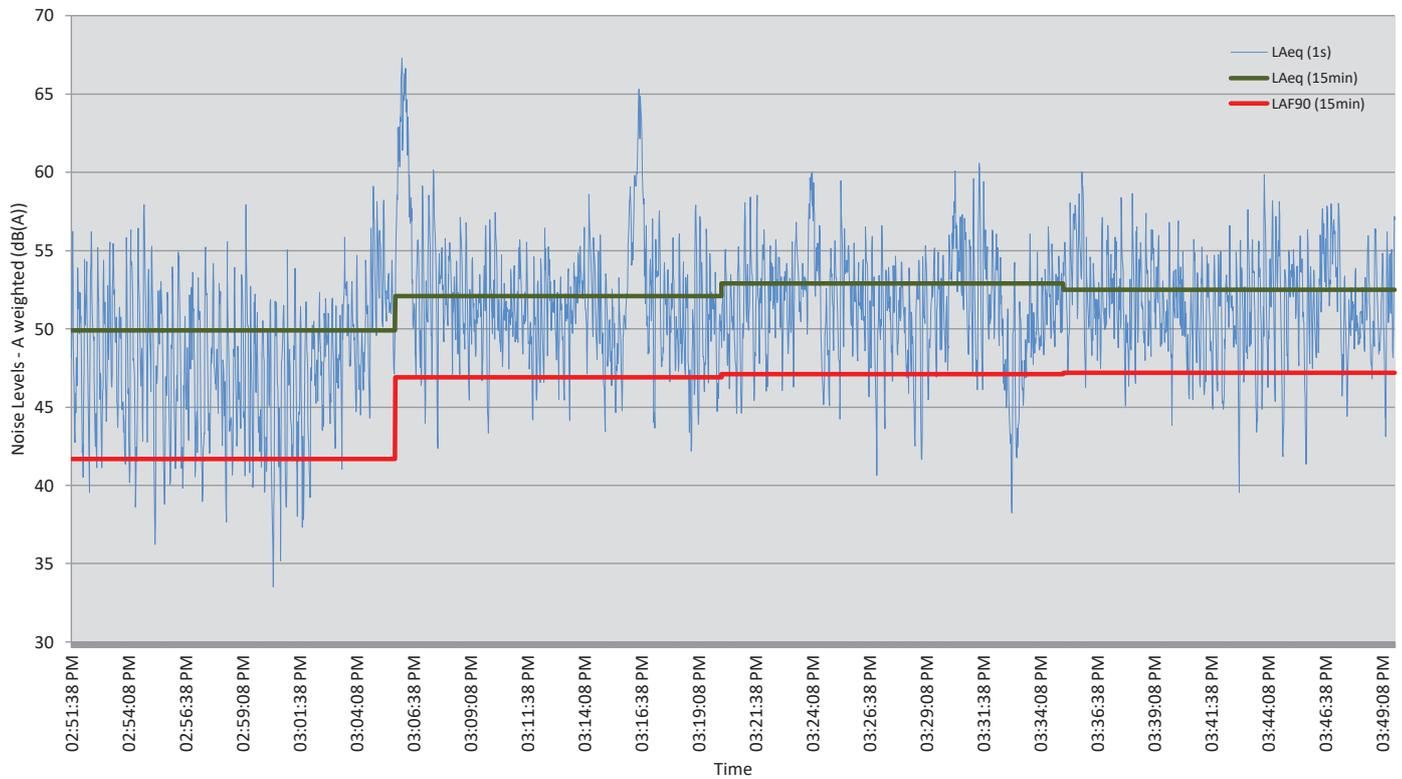
Pakiri Sand Extraction - Noise Level Measured at Position 6 - 22<sup>nd</sup> May 2019
