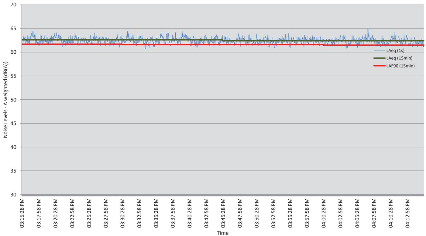
Pakiri Sand Extraction - Noise Level Measured at Position 3 - 07<sup>th</sup> May 2019
