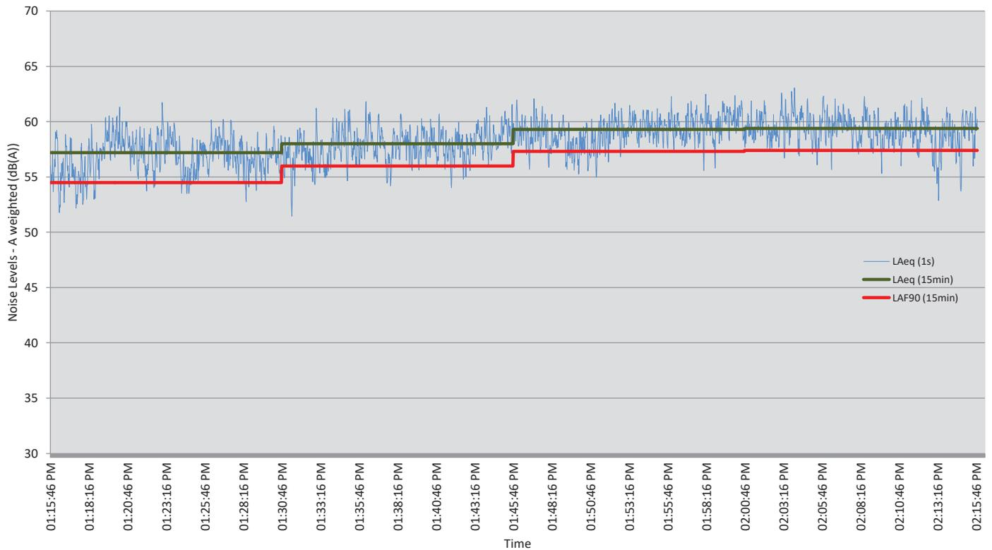
Pakiri Sand Extraction - Noise Level Measured at Position 2 - 13<sup>th</sup> June 2019
