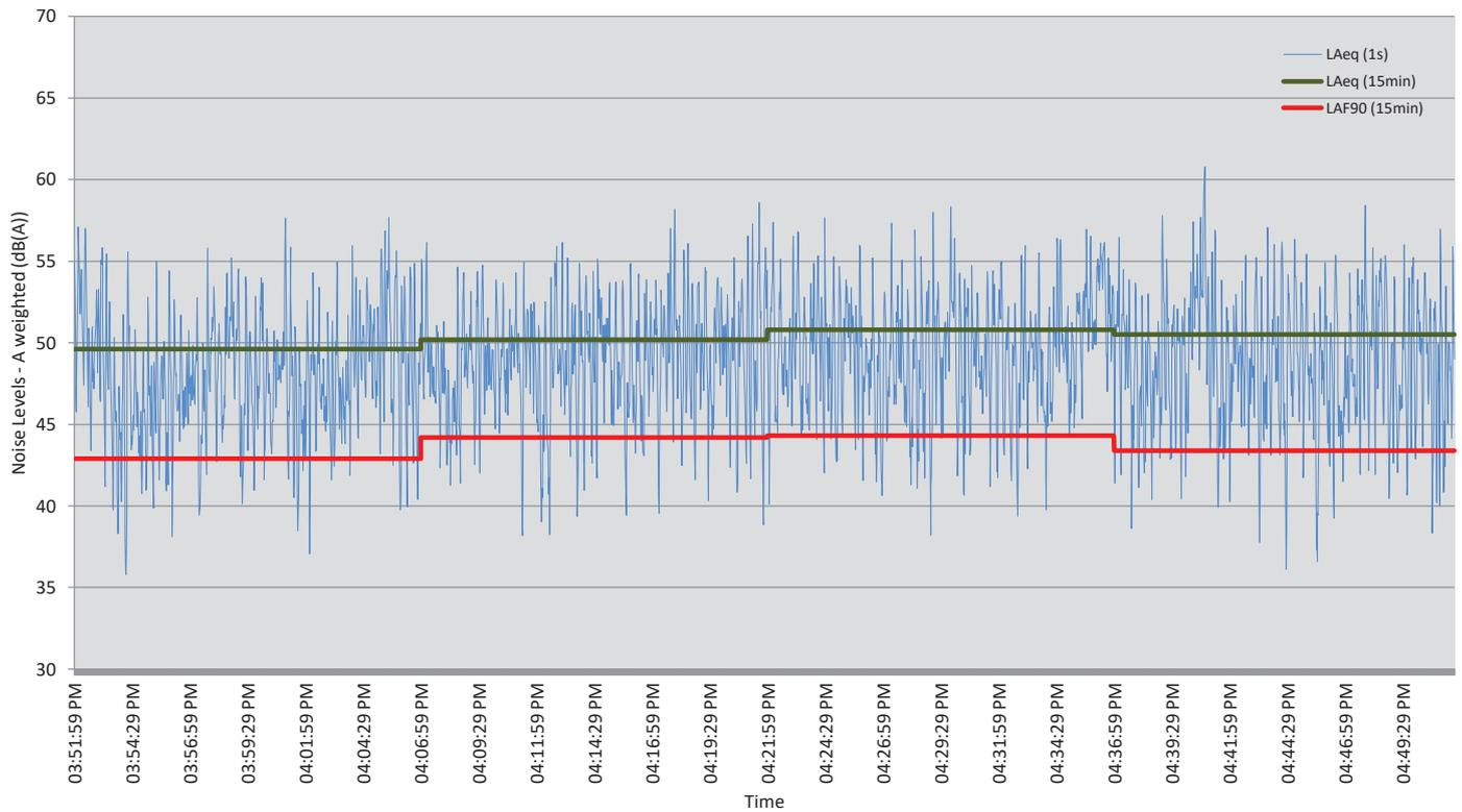
Pakiri Sand Extraction - Noise Level Measured at Position 1 - 13<sup>th</sup> June 2019
