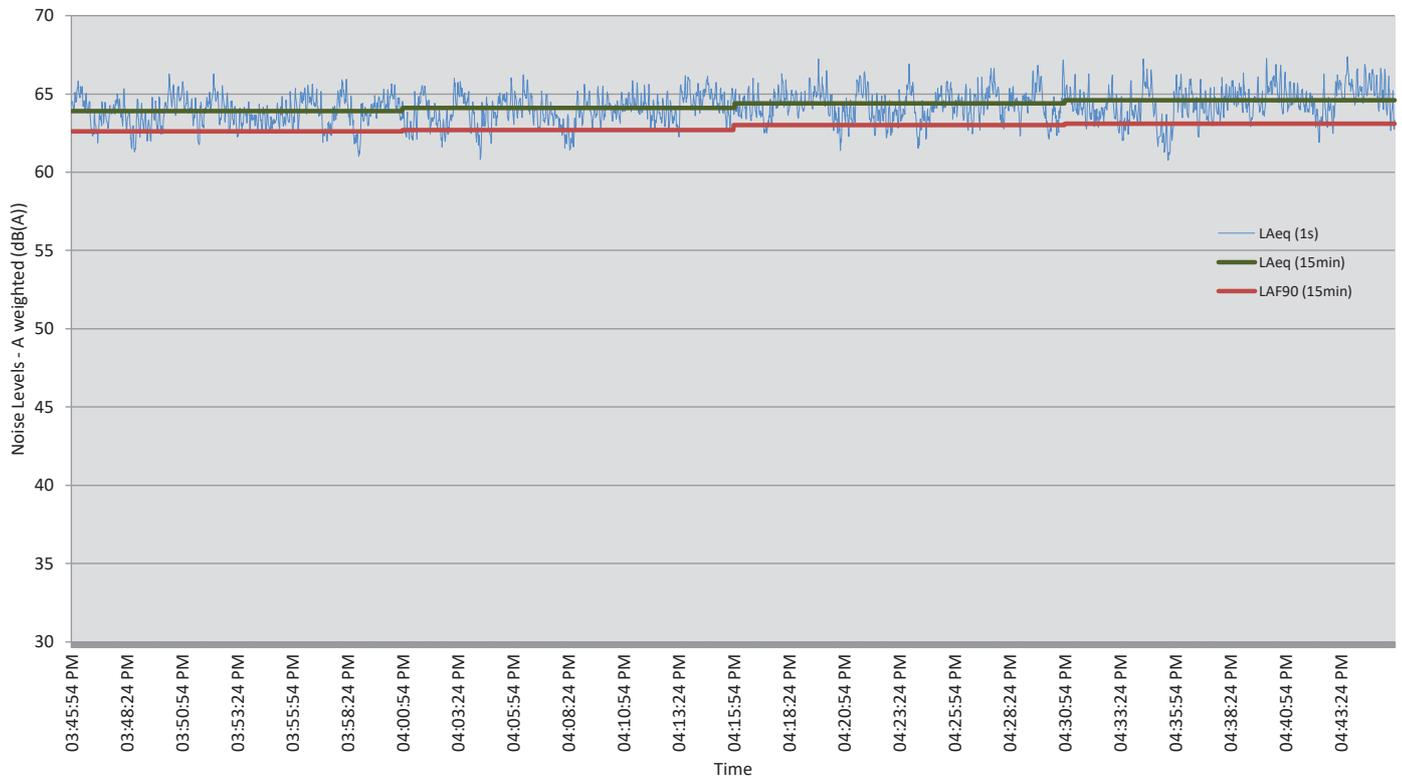
Pakiri Sand Extraction - Noise Level Measured at Position 2 - 03<sup>rd</sup> May 2019
