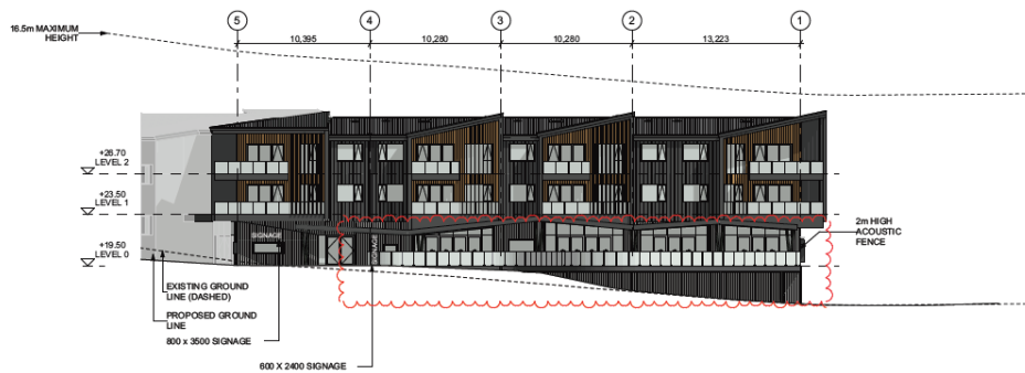
Figure 11: Eastern elevation of Block G
