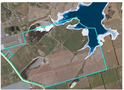
The bulk of the WWTP even at full build out as can be seen from the Indicative Design and Operational Report is avoiding the area shown as subject to the 1 in 100-year return at both 1 m and 2 m sea level rise.
