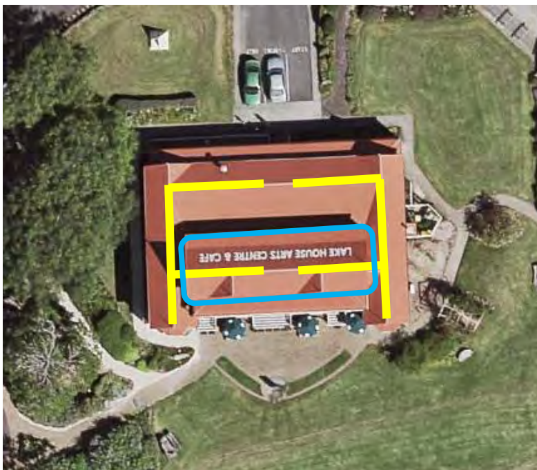
Figure 3: Diagram illustrating how the Lake House is believed to have been developed with two mirrored F-plan villas (yellow) and a second storey addition (blue)
