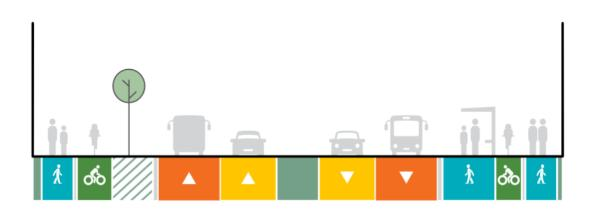
Figure 8-33: Indicative design between Postman Road and the new Wilks Road Interchange – 30m cross section
