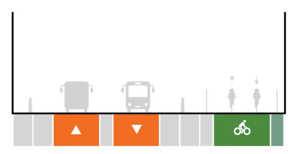
Figure 8-4: Rapid transit corridor – indicative 20m cross section
