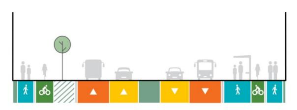
Figure 8-24: Silverdale interchange to Wilks Road; and Richards Road to Durey Road (4 lane urban arterial, 30 m)
