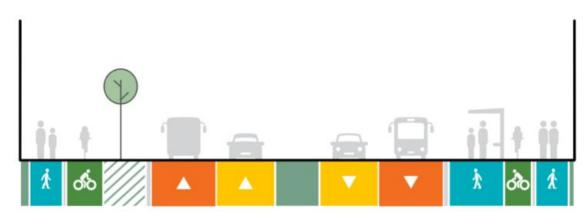
Figure 8-35: Indicative design – 30m four lane cross section
