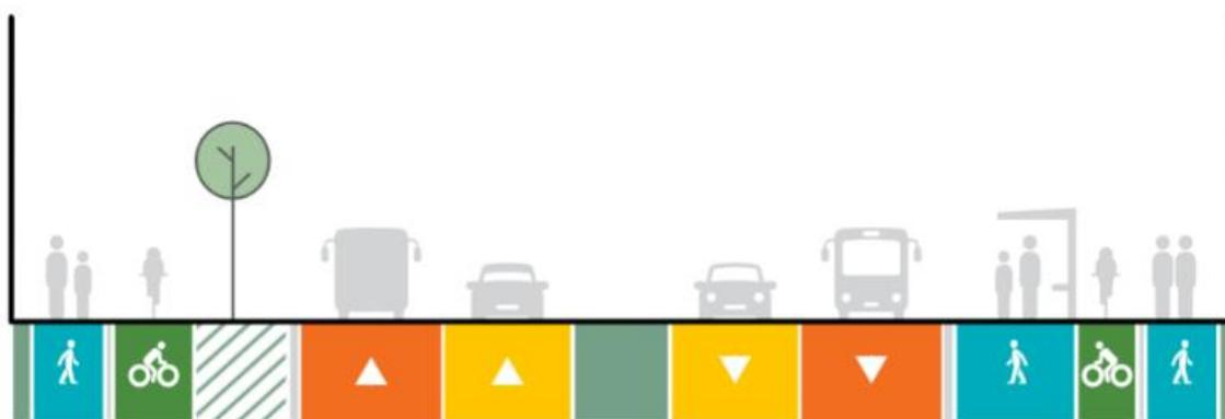
Figure 8-35: Indicative design – 30m four lane cross section
