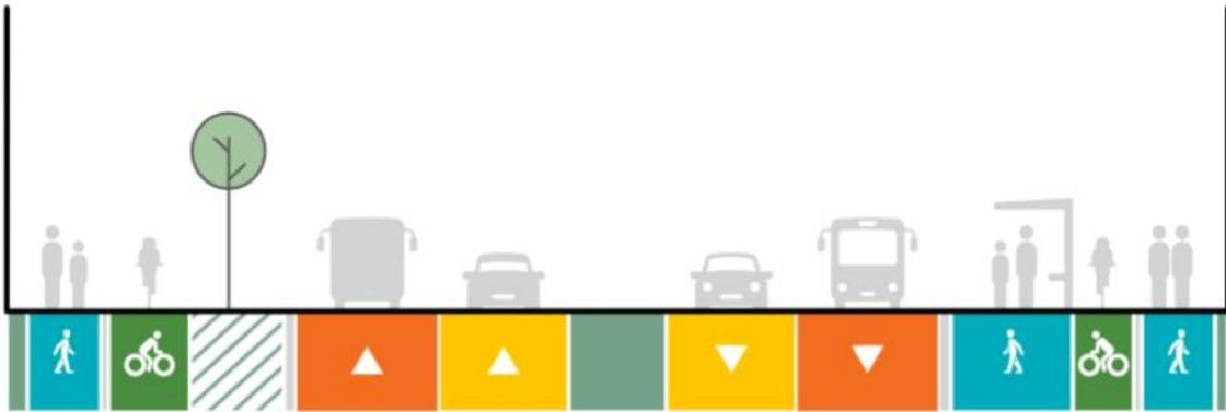
Figure 8-24: Silverdale interchange to Wilks Road; and Richards Road to Durey Road (4 lane urban arterial, 30 m)
